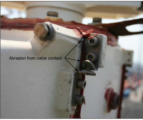
Figure 19: Additional contact marks on the radar scanner
