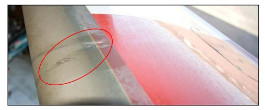
Figure 13: Contact marks on the tail rotor
