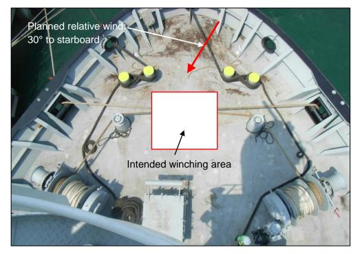
Figure 4: Planned winching area<sup>9</sup> and relative wind
