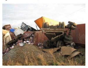
At the time of the accident the area surrounding the level crossing was enveloped in very thick fog, with visibility less than 50 m. The investigation found that the truck was not being driven in accordance with these conditions, and that the performance of the truck driver may have been affected by fatigue. In addition, the level crossing approach signage and sighting distances were not in accordance with the relevant Australian standards.
