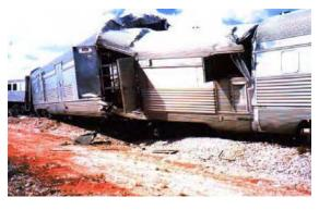
Three months later, on 26 November 1999, a similar accident occurred at Ararat in Victoria. A rail employee wrongly moved the points and diverted a grain train into the Ararat yard, where it collided with a stationary ballast train. Two train crew members were seriously injured. Given that it was possible to move the points in front of an oncoming train, the ATSB led investigation determined that the system in operation at Ararat was fragile in the face of human error.
