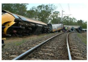
The principal cause of the derailment was excessive speed. From a systemic point of view, the accident was complex and although the principal causal factor related to 'human performance', better organisational controls may have prevented it.
