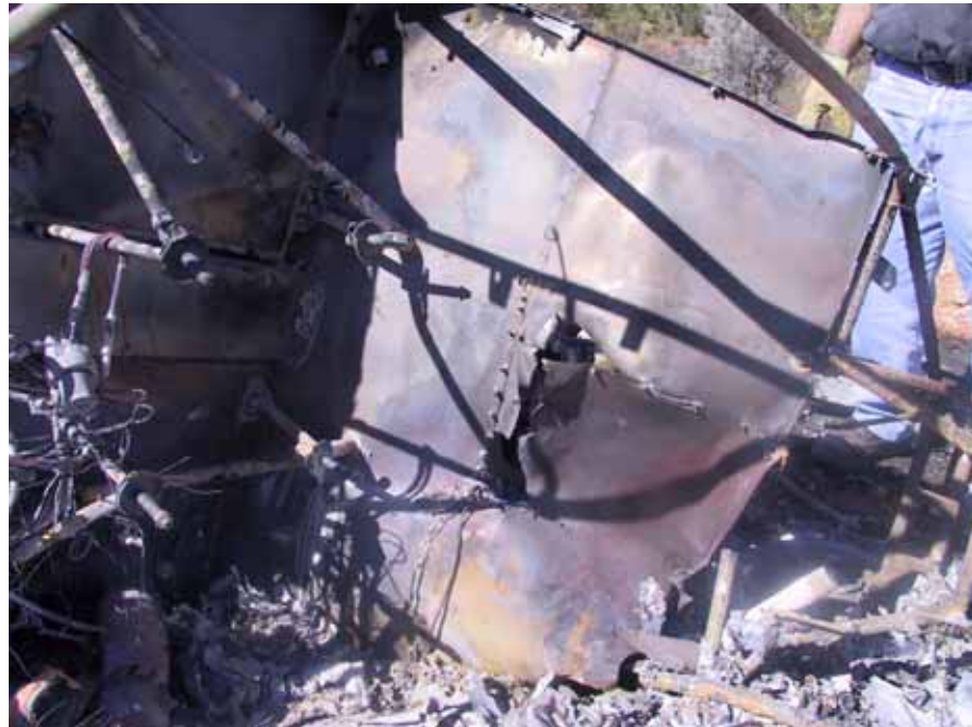
Figure 5: Flex plate puncture of stainless steel firewall above engine.
