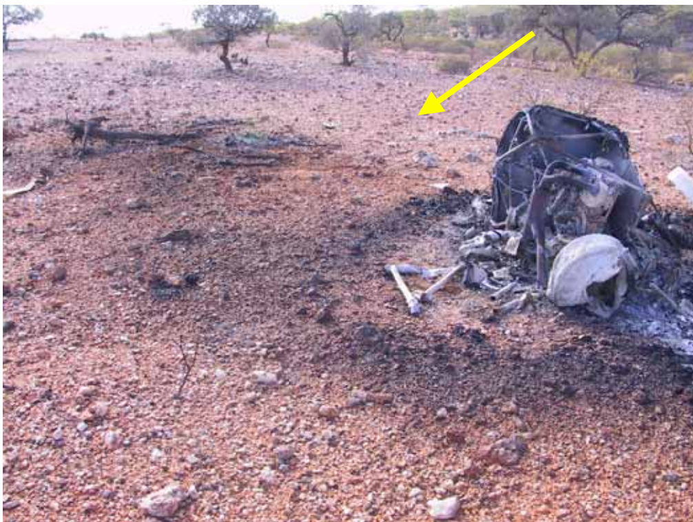
Figure 6: Sooting pattern adjacent to wreckage (arrow indicates approximate direction of flight at impact)
