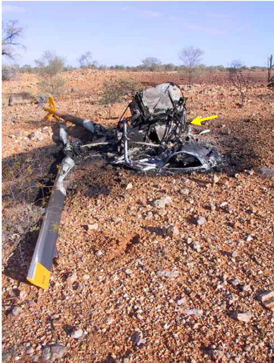
Figure 1: Helicopter wreckage (arrow indicates bulkhead deformation behind pilot seat position)
