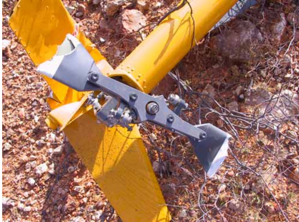
Figure 2: Tail rotor damage
