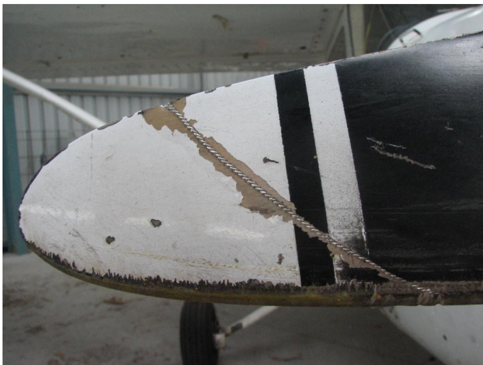
Figure 8: Propeller damage and wire imprint
