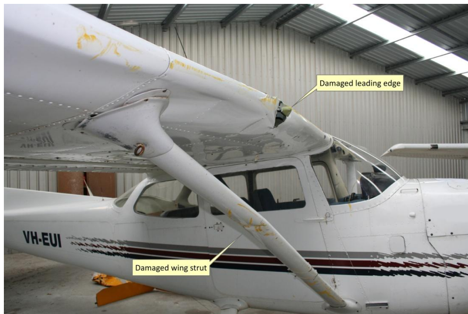
Figure 7: Damage to VH-EUI's right wing and strut
