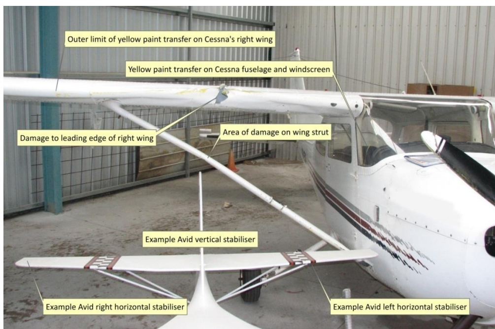
Figure 11: Alignment of an exemplar Avid with the damage to EUI
