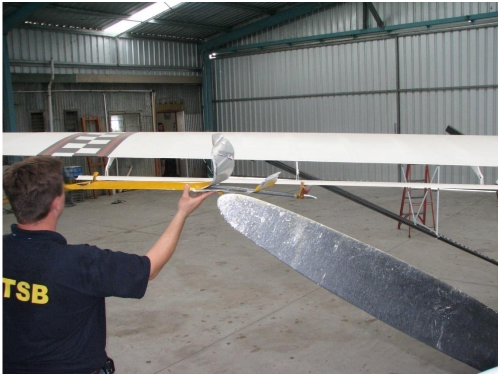
Figure 12: Reconstructed alignment of the Avid's damaged left flaperon and EUI's propeller arc
