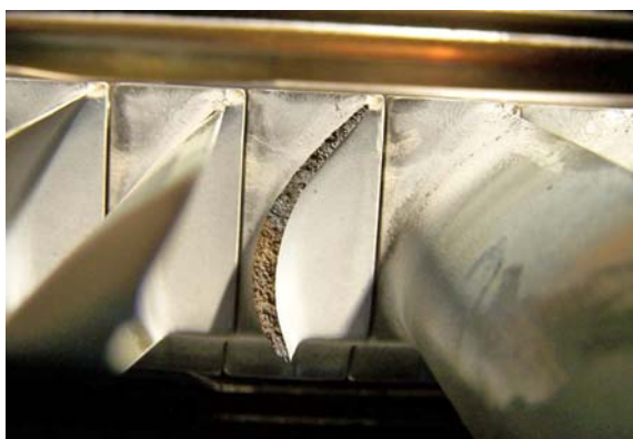
Figure 3: Fractured stage-four PT blade (SN R4PUA)
