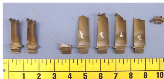
Figure 1: Separated and damaged stage-four PT blades
