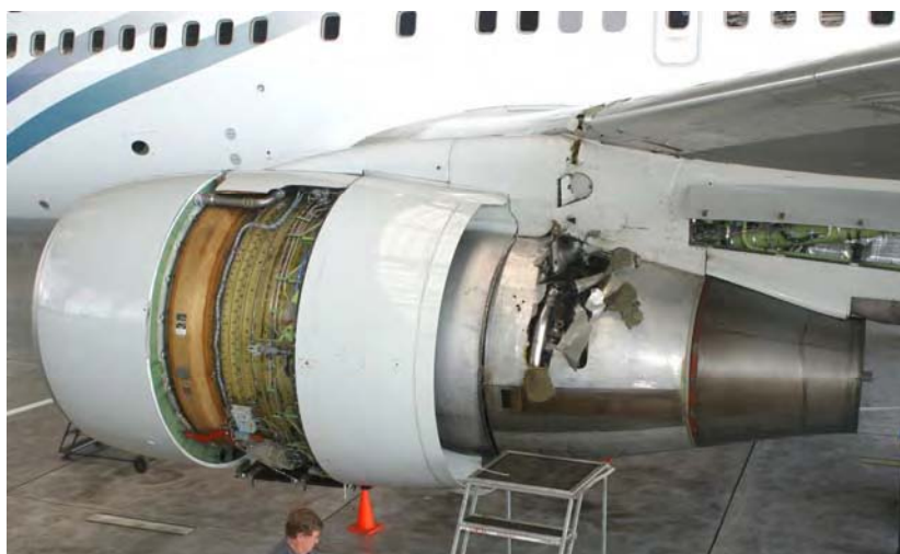
Fig. 1 Failed left (No.1) engine from Boeing 767-219 ZK-NBC.
