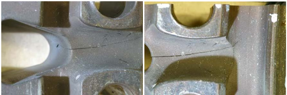
Figs. 15 & 16 Rear-face view of the cracking found within fir tree slot 72.
