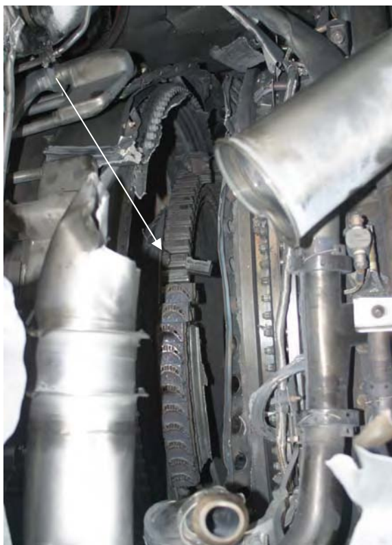
Fig. 4 View of the stage-1 HPT disk through the severed case. Many blades fractured or lost from the disk.
