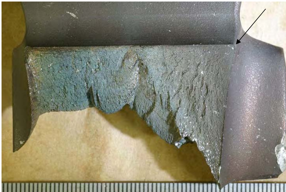
Fig. 12 Closer view of the primary fracture origin. Note the absence of characteristic fatigue propagation marks, attributed to crack growth by an intergranular propagation mode.
