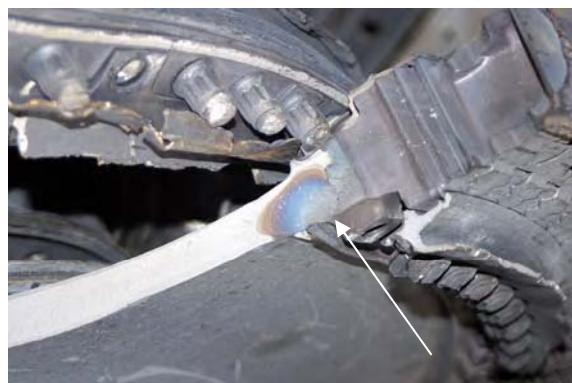
Fig. 6 Primary disk fracture showing an area of discoloured prior cracking at the base of a blade firtree slot.
