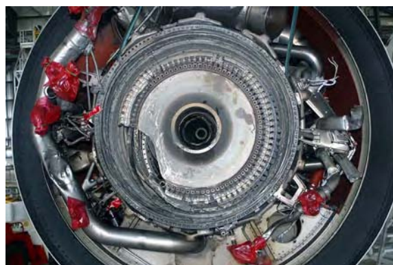
Fig. 5 Rear face of the stage-1 HPT disk, showing the loss of the rim and web section.
