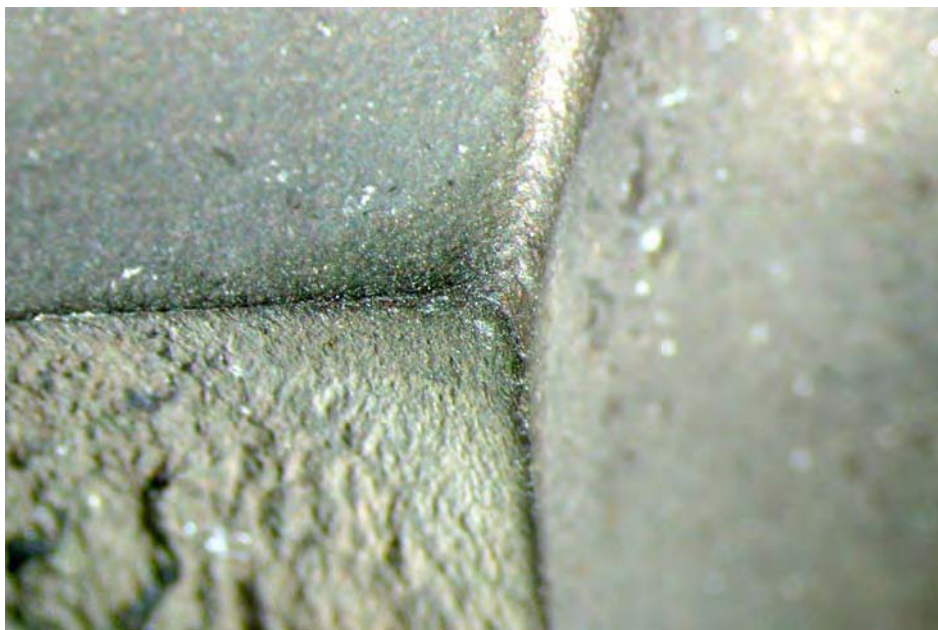
Fig. 13 Low-power microscopic view of the crack origin. The surrounding slot, corner and rear faces appeared free of damage at that magnification.
