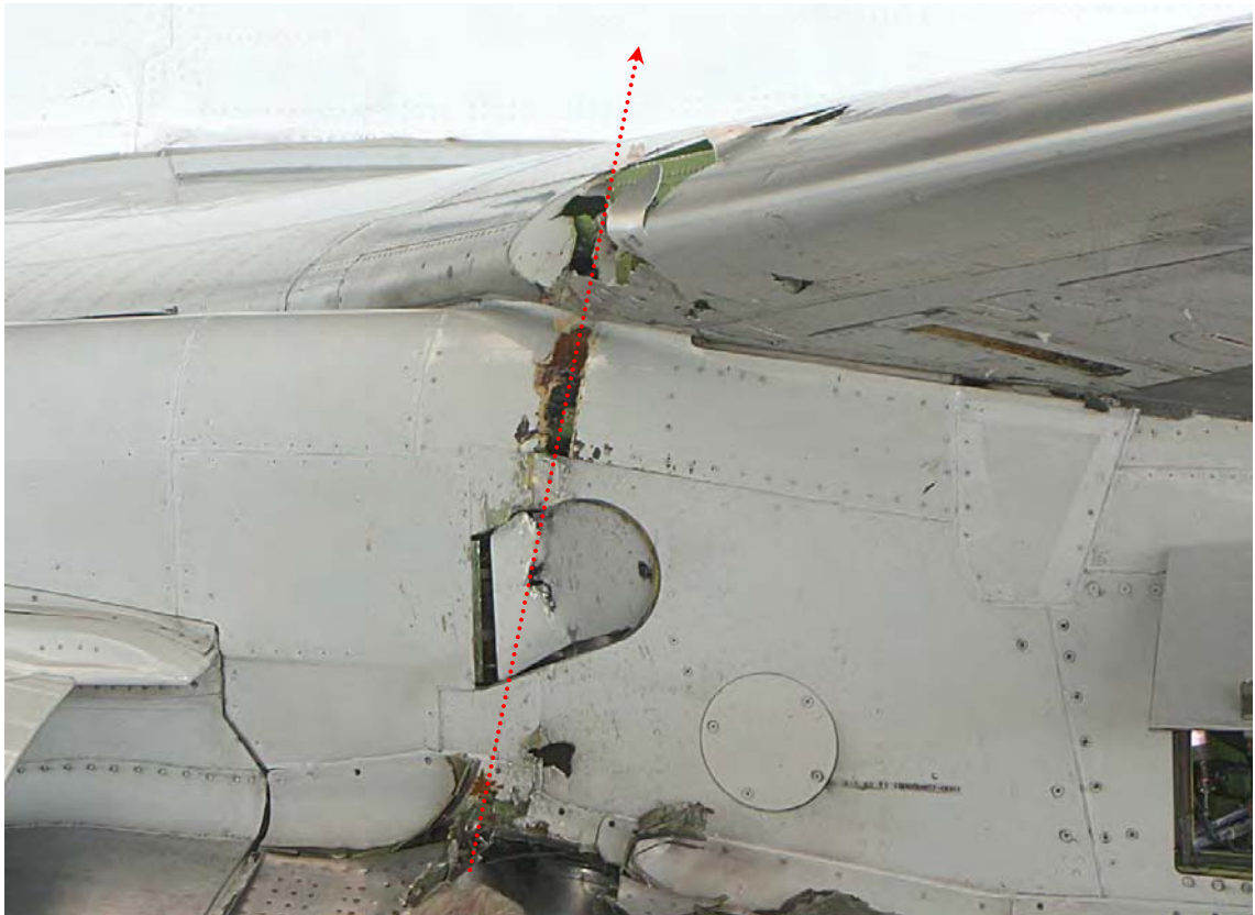
Fig. 2 Vertical gouge in the engine pylon fairings – likely produced by the liberated segment of high-pressure turbine disk. The dotted line illustrates the likely trajectory of the disk fragment.
