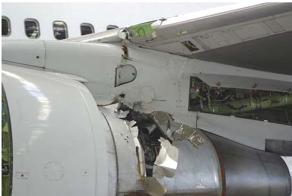
Fig. 1 Overview of the damage sustained by the left engine and wing leading edge of ZK-NBC
