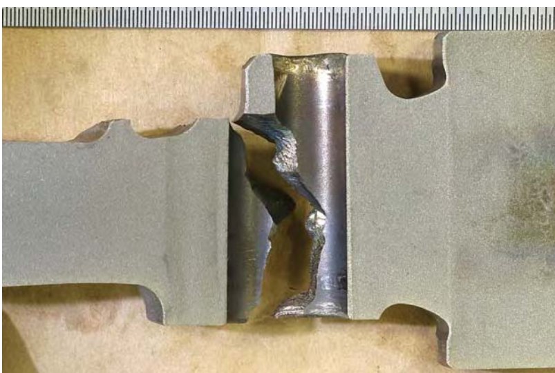
Fig. 11 Wire-cut surfaces of the specimen above, showing the divergence of the primary fatigue cracking into the rim bolt hole.
