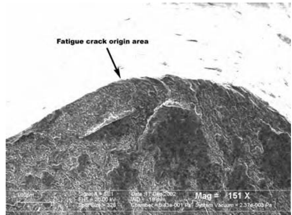
Fig. 33 Crack origin again identified at the rear break-edge tangency point.
