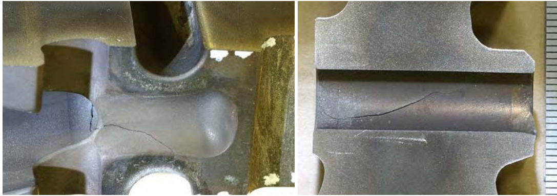
Figs. 17 & 18 Forward face and internal bolt hole views of the slot 72 cracking.
