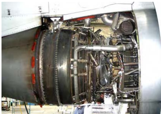
Fig. 2 Core damage to the engine around the plane of the first-stage high-pressure turbine disk.
