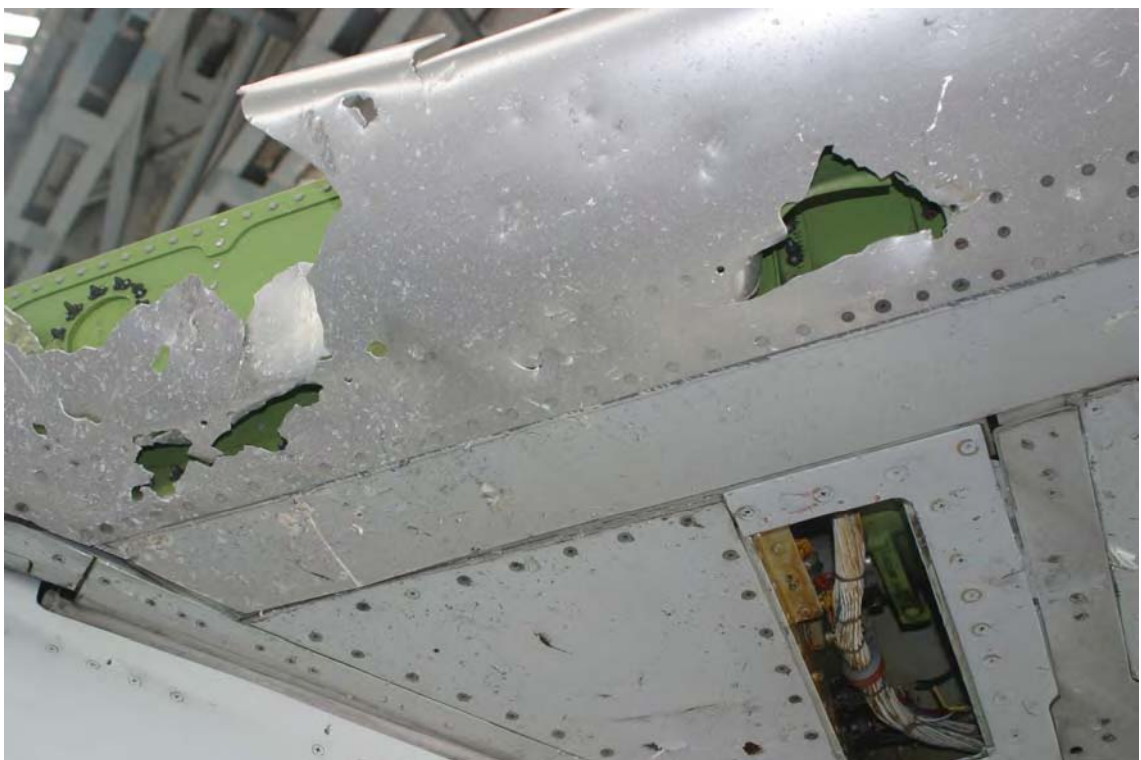
Fig. 3 Damage to the wing leading edge profile above the engine core rupture.
