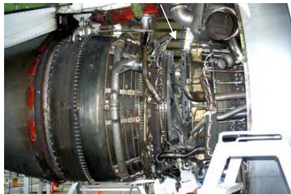
Fig. 3 Separation of the engine core (arrowed).
