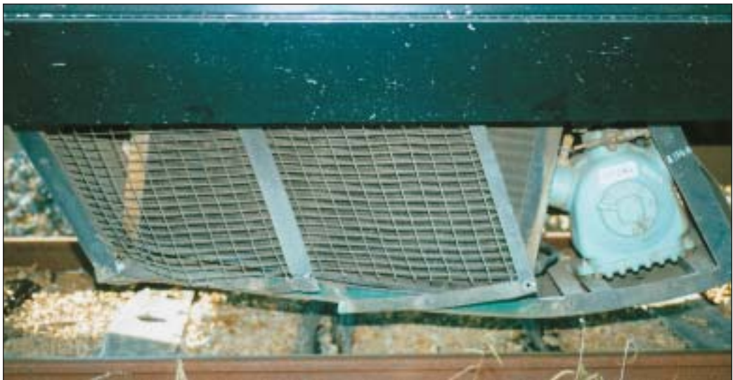
FIGURE 5: Damaged refrigeration units under carriage
