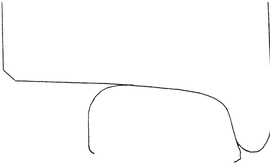
FIGURE 25: Predicted number-1 wheel contact with high rail
