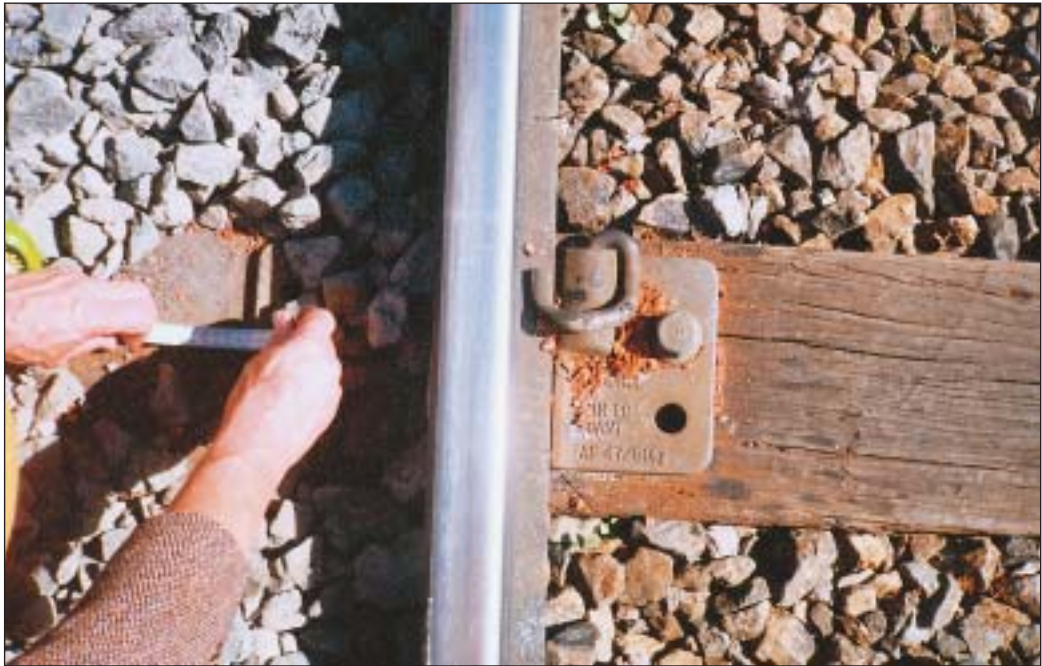
FIGURE 19: Measuring plate movement on a Pandrol fastening fitted to the high rail the point of derailment
