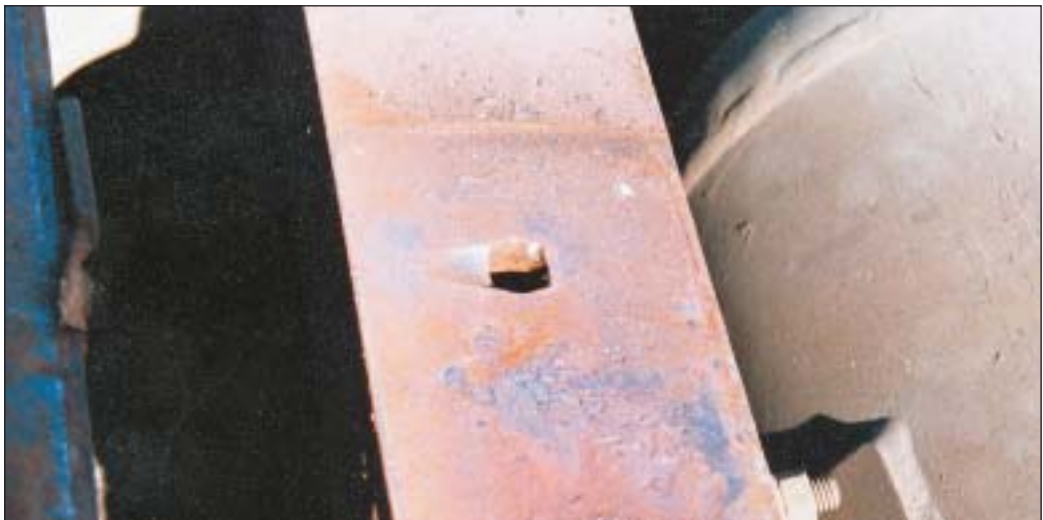
FIGURE 6: Side bearer mounting surface on bogie bolster showing deformation around locating hole
