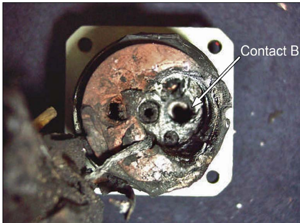
Figure 9: Comparison of electrical terminal block connector pins: burnt pin B from VH-EBF (lower) and that from an exemplar unit (upper)
