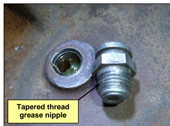
Figure 10: View of grease nipple removed showing tapered thread
