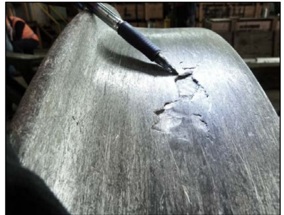
Figure 7: Surface defect in 2L wheel
