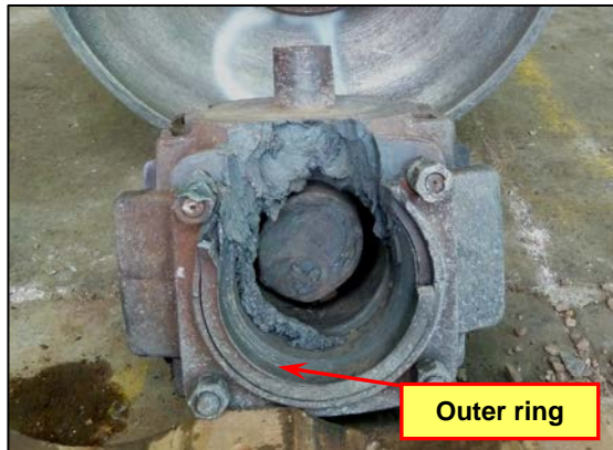
Figure 5: View inside failed '2L' axle-box with the screwed part axle journal remaining
