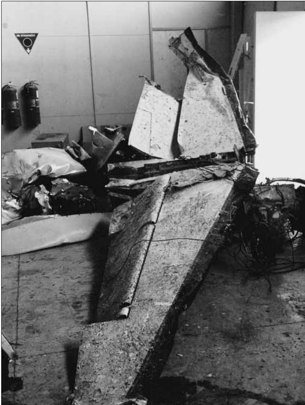
Figure 6. Left tailplane exhibited damage consistent with high speed water impact. Rudder (removed) and elevators showed no evidence of inflight failure.
