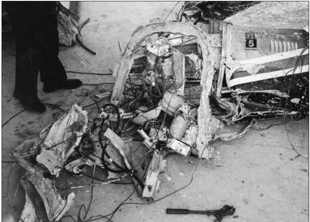
Figure 5. Shattered rear fuselage as recovered from sea.
