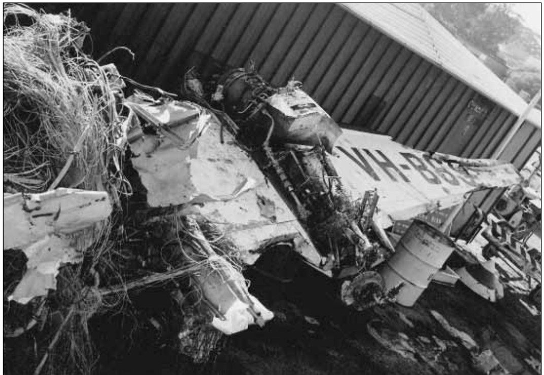
Figure 4. View of left wing (inverted). Crush damage to outer leading edge consistent with high speed water impact.
