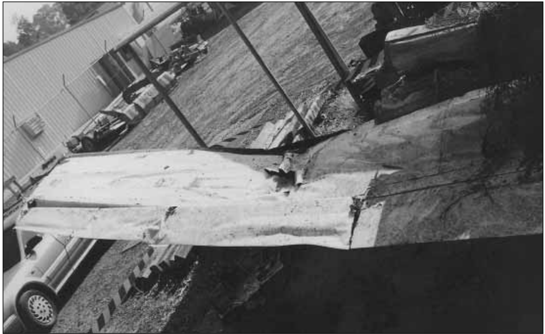
Figure 3. Right aileron (inverted) showed no evidence of 'flutter' or 'snatch'.
