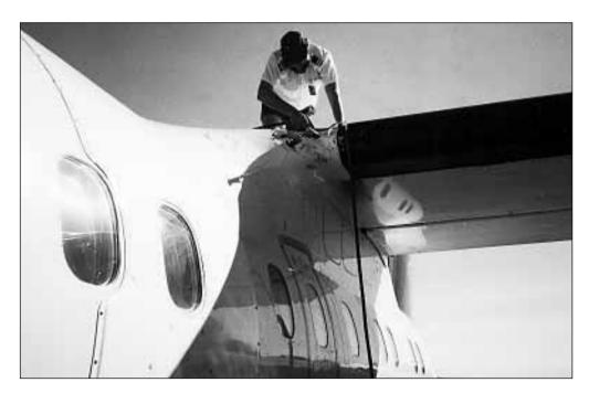
Figure 2. Damage at wing-fairing to fuselage.
