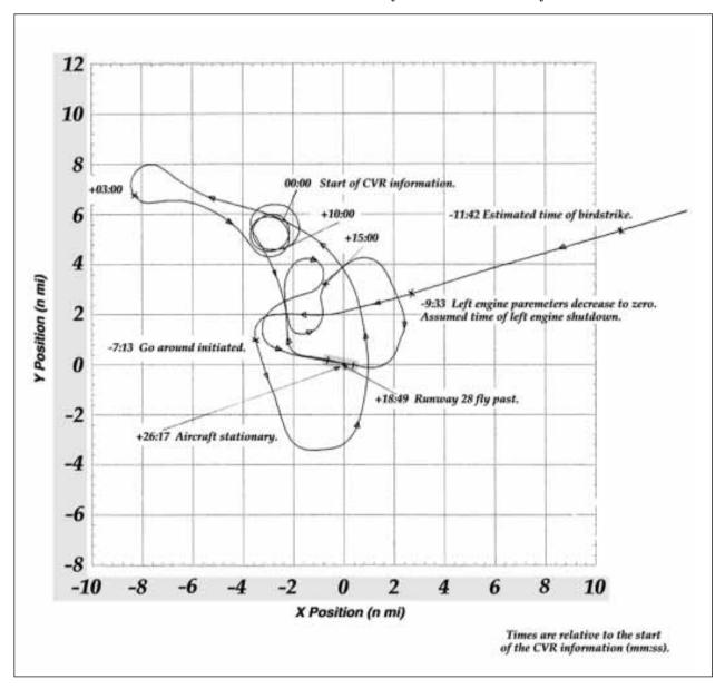
Figure 1. Derived ground track of VH-JSI
