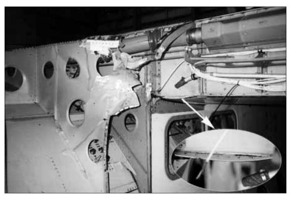
Figure 3. Damage to main spar and associated components.
