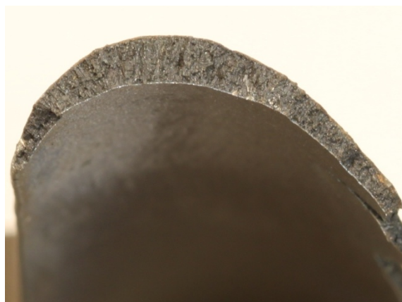
Figure 5: Typical appearance of blade fracture surfaces
