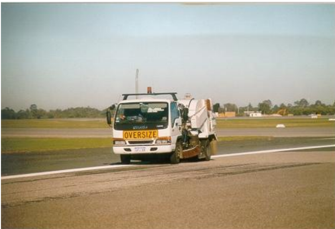
FIGURE 1: Runway sweeper vehicle
