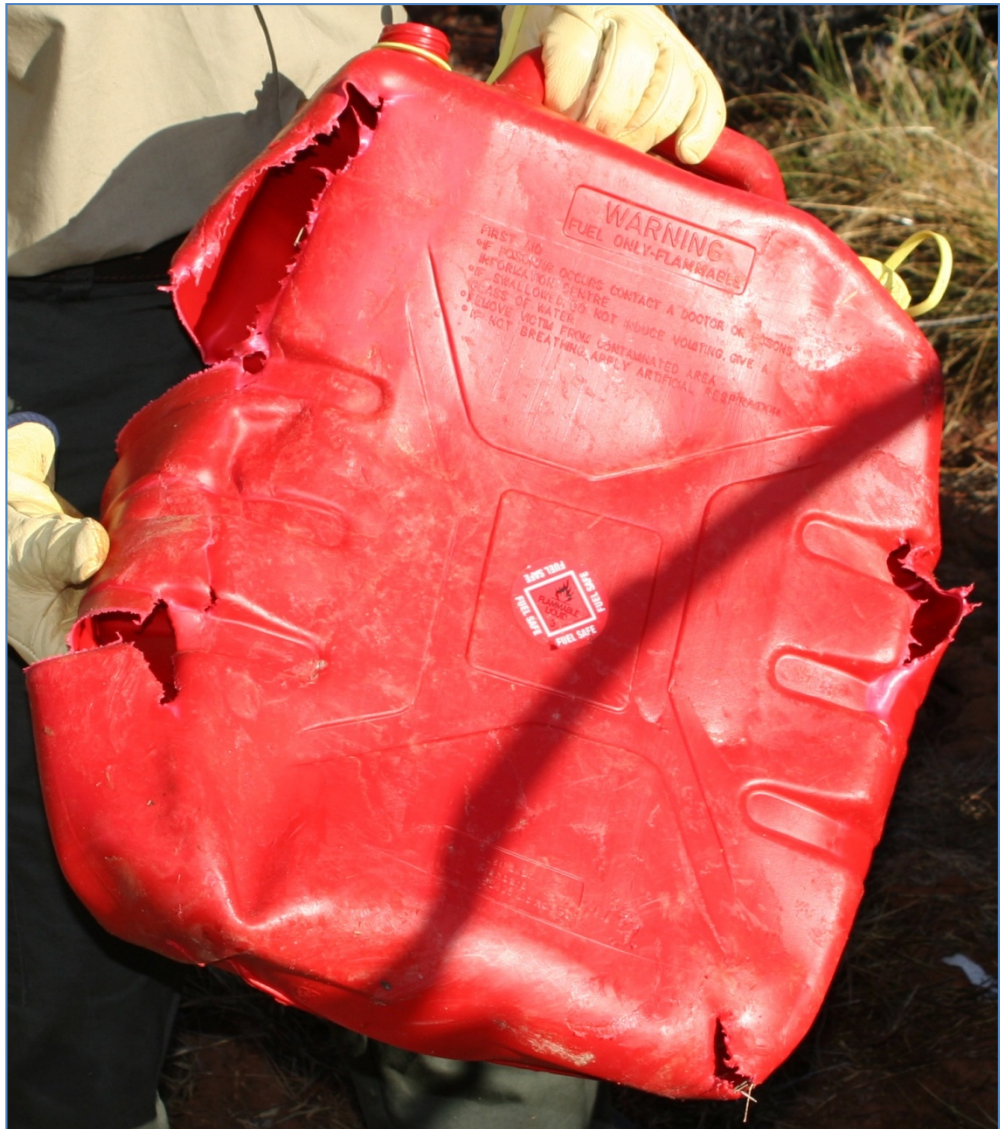
Figure 14: Burst fuel container
