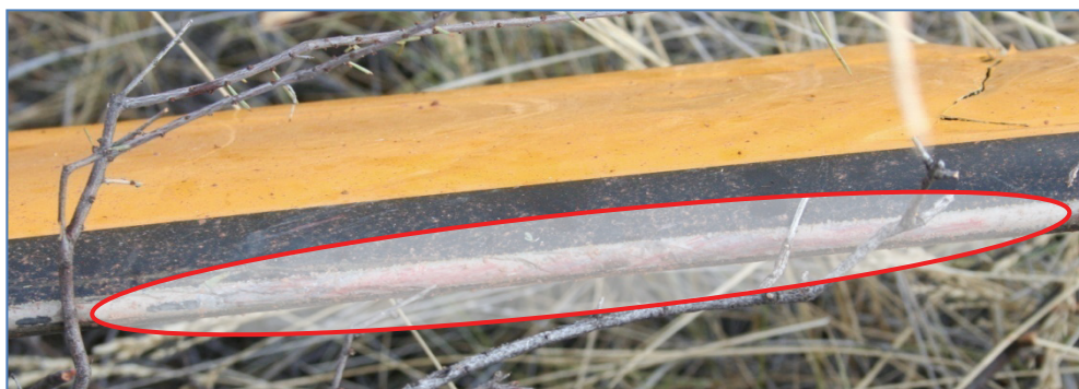
Figure 5: Red paint transfer onto the leading edge of the main rotor blade
