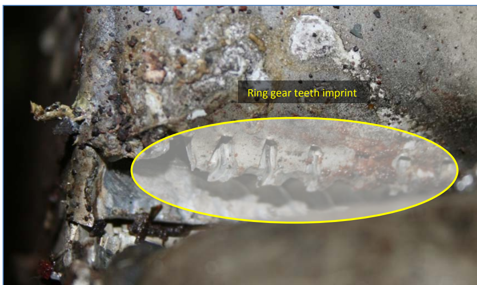
Figure 9: Static ring gear teeth imprint on the engine oil cooler
