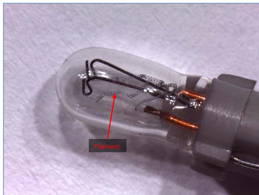
Figure 11: Instrument lamp displaying filament stretch
