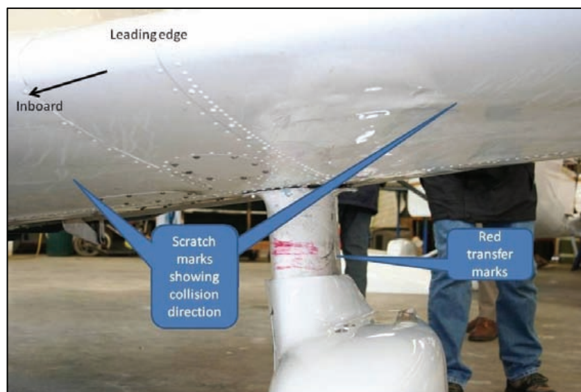
Figure 8: Scratches and wiring insulation transfer marks on CGT's left wing and landing gear
