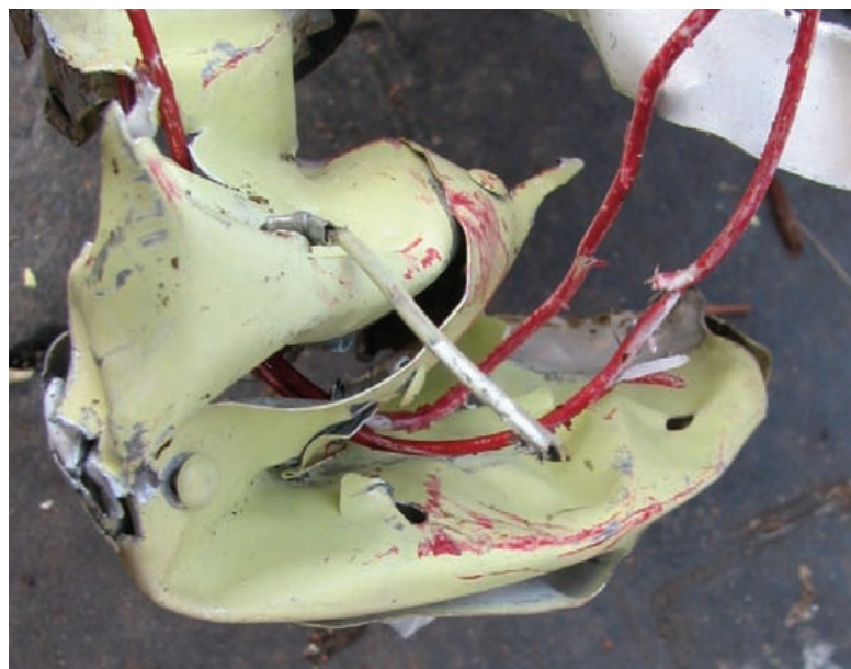
Figure 9 Damaged red electrical insulation from UPY's left wing
