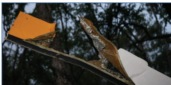
Figure 2: Main rotor blade damage 5
