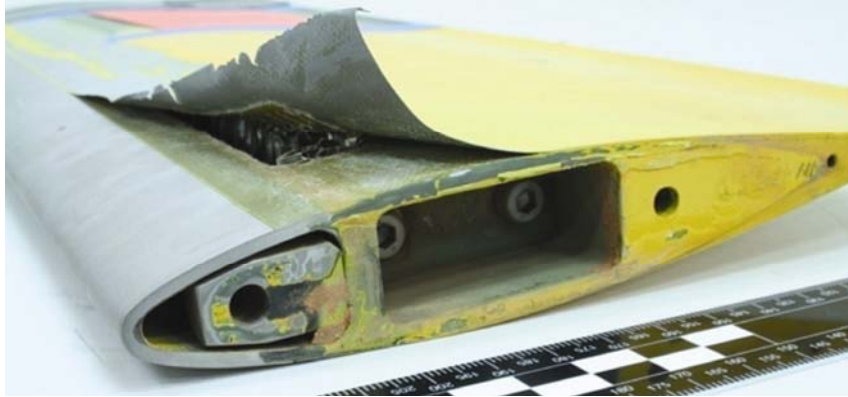
Main rotor blade skin debonding (AO-2009-002)
