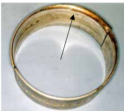
Figure 3. Connecting rod bearing shells from the number-four assembly. The outward splaying of the forward edge is clearly visible (arrowed).
