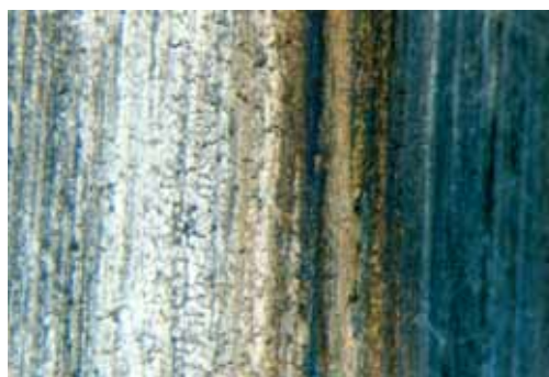
Figure 2. Internal surface of a fragment of the cylinder liner – shows very similar characteristics to the piston skirt.
