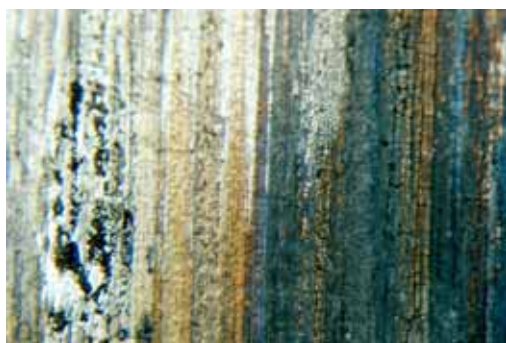
Figure 1. External surface of a fragment of the piston skirt – shows appreciable axial scoring and frictional heat tinting.
