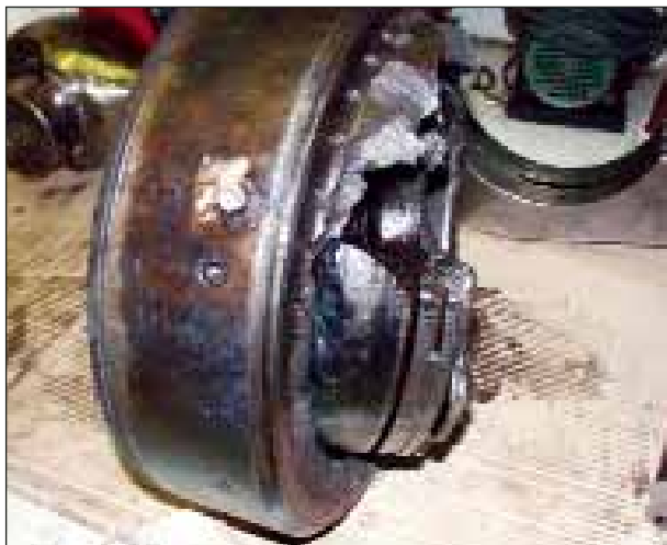
FIGURE 4: Top of cylinder liner with remains of piston crown jammed within it
