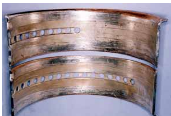
Figure 4. Internal (running) surfaces of the bearing shells illustrating the forward edge damage and the wiping of the surface white-metal layer.
