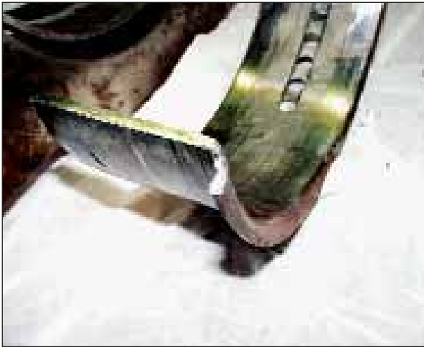
FIGURE 5: Front edge of upper half of bottom-end bearing shell splayed back in way of crank web
