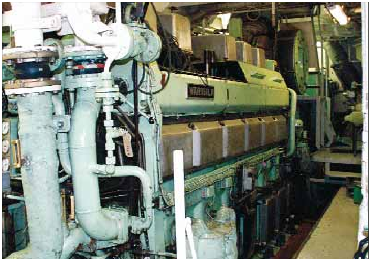
FIGURE 3: Main engine of ANL Purpose – Wärtsilä Vasa GR32 four-stroke diesel
