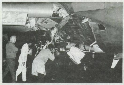
FIG. 1 Damage to VH-TJA in forward wing root area on starboard side. The arrow indicates the point of first contact.
