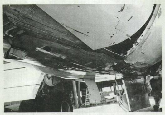
FIG. 3 Underside of fuselage of VH-TJA showing score marks and punctures between starboard wheel bay area and tail bumper.
