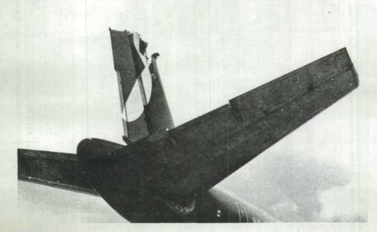
FIG. 4 Damage sustained by tail fin and rudder of CF-CPQ.
