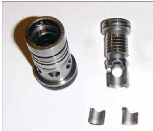
FIGURE 11: Broken stop valve pieces
