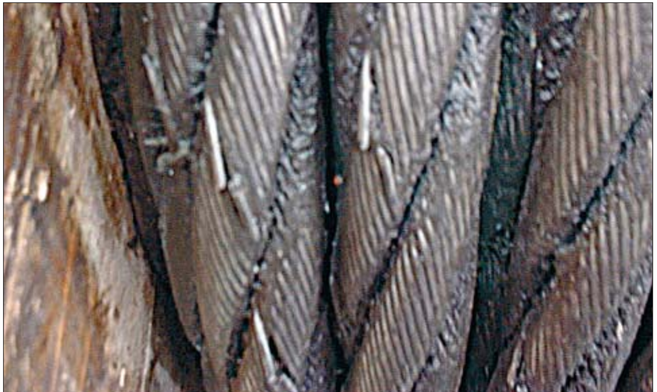
FIGURE 3: Wire from No. 2 crane showing breaks within strands
