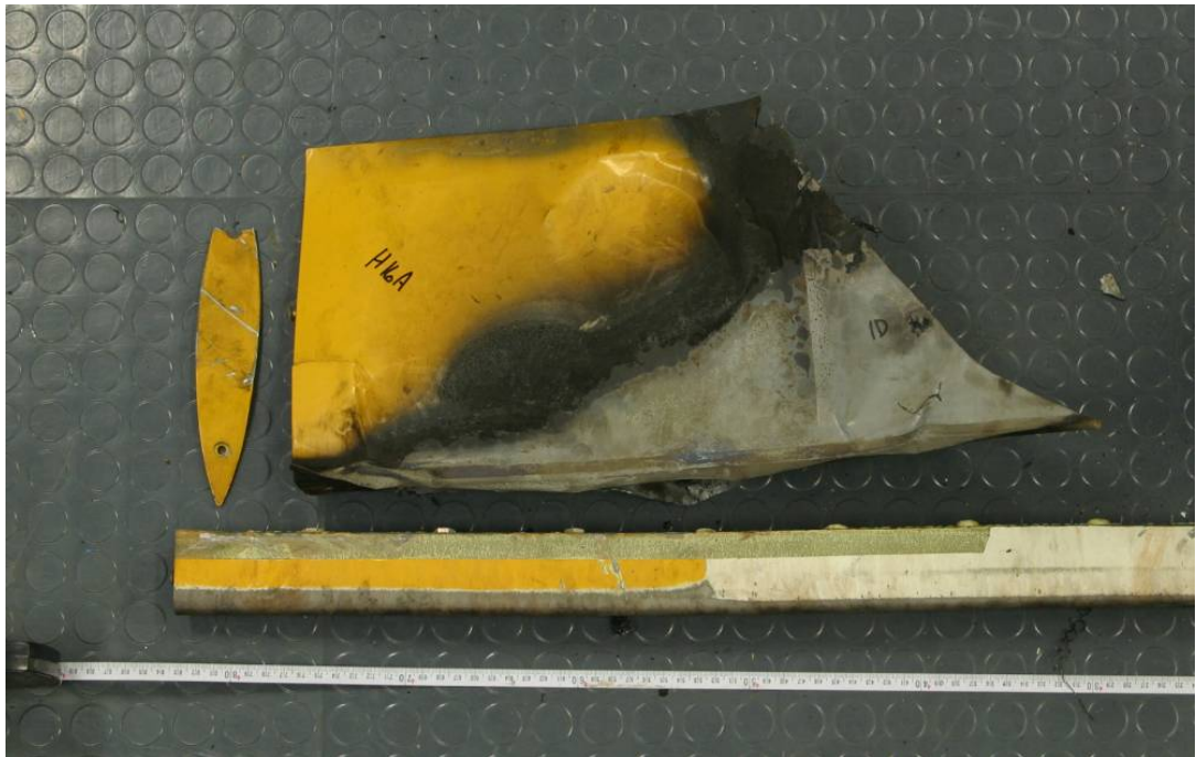
Figure 2: Area at the tip of blade S/N 4202-A that exhibited backward peeling separation of the skin from the leading edge spar.
