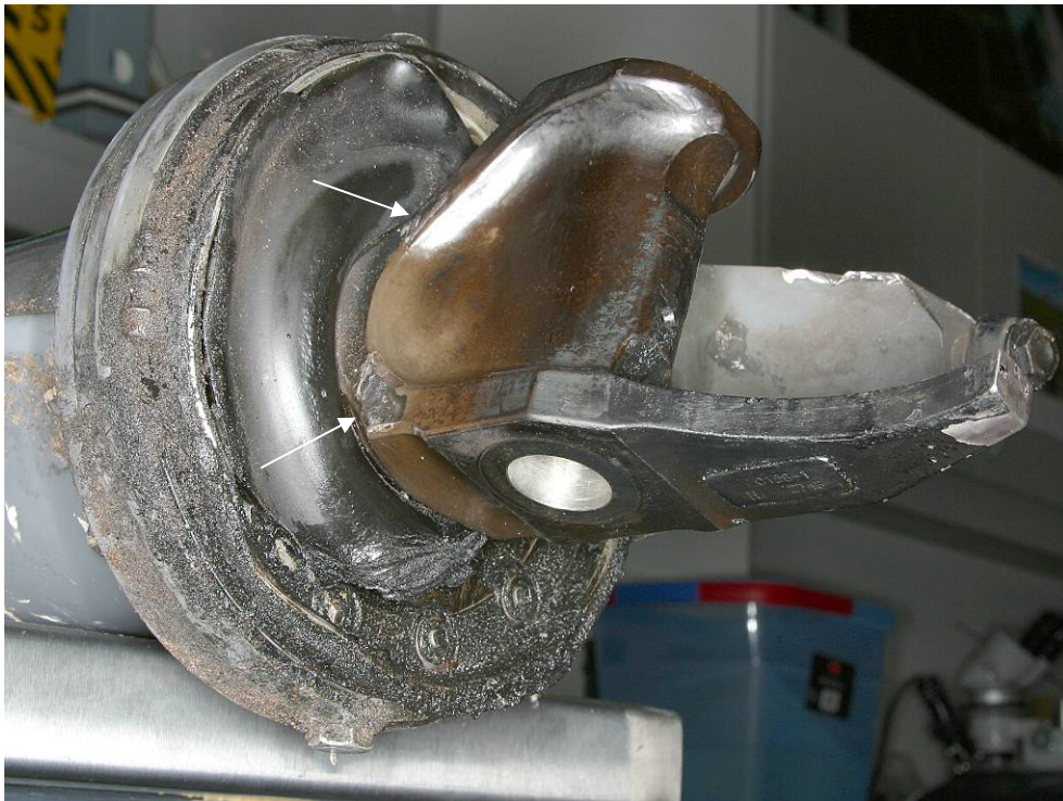
Figure 3: Hub assembly of blade S/N 4202-A – contact against the up-coning stop shown at arrows.
