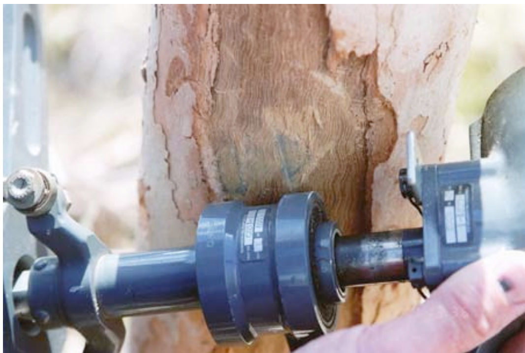
Figure 3: Tail rotor gearbox assembly tree imprint
