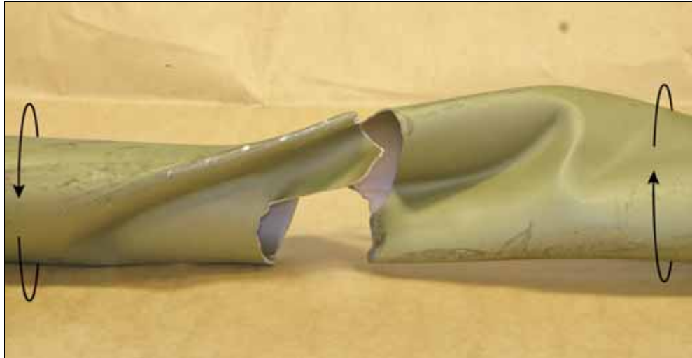
Figure 5: Various external secondary surface damage including scratches, rotational scuff marks and indentations were observed along the length of the shaft.
