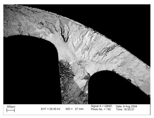
Figure 5: Detailed view of the boundary between the planar defect and fatigue cracking
