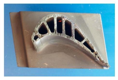
The site of fatigue initiation is arrowed
