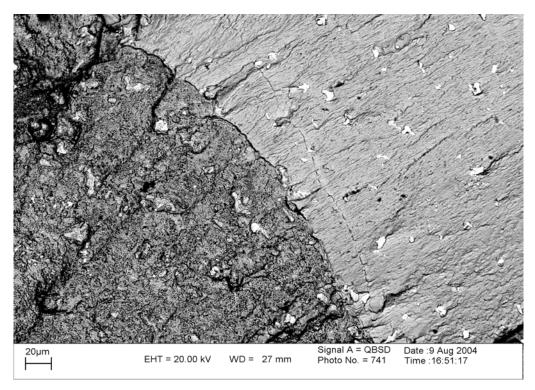
The region of fatigue crack propagation is to the right
