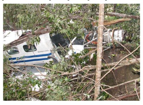
Examination of the aircraft wreckage accounted for all major parts of the aircraft, including all flight control surfaces on-site. Continuity of the flight control systems was established. All fracture surfaces showed evidence of impact overloads and there was no evidence of fatigue cracking, corrosion or any pre-existing defect. There was no evidence of any pre-existing defect with the aircraft that would have contributed to the accident.
