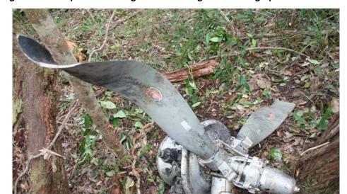
Figure 7: Propeller showing blade bending and missing tip section
