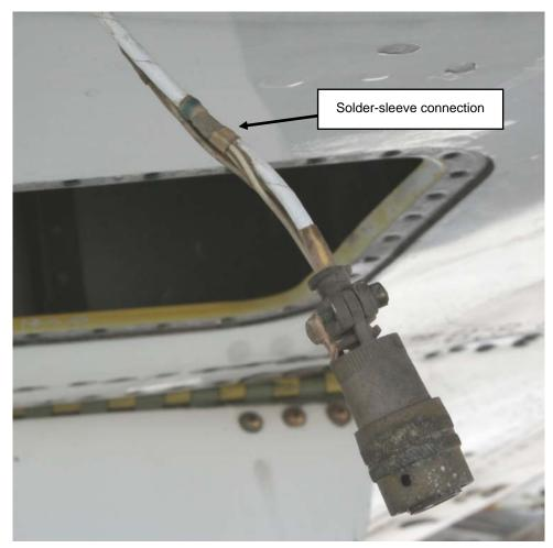
Figure 3: Typical solder-sleeve connection
