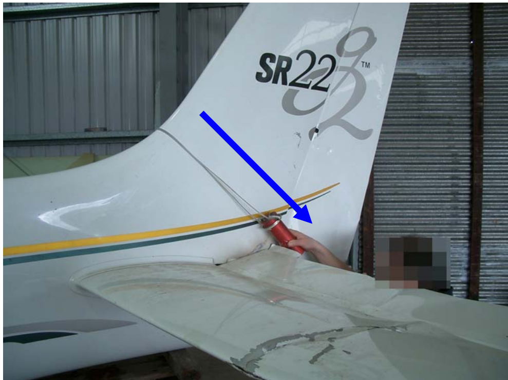
Figure 15: Path travelled by the CAPS rocket and harness
