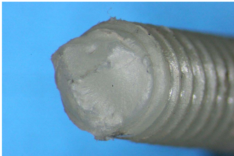
Figure 19: Conical fracture surface of nylon tension screw A
