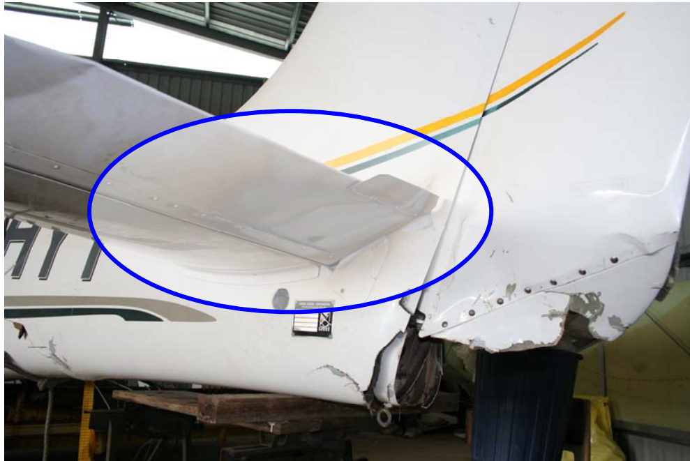
Figure 16: Burnt paint (circled) on lower surface of left elevator
