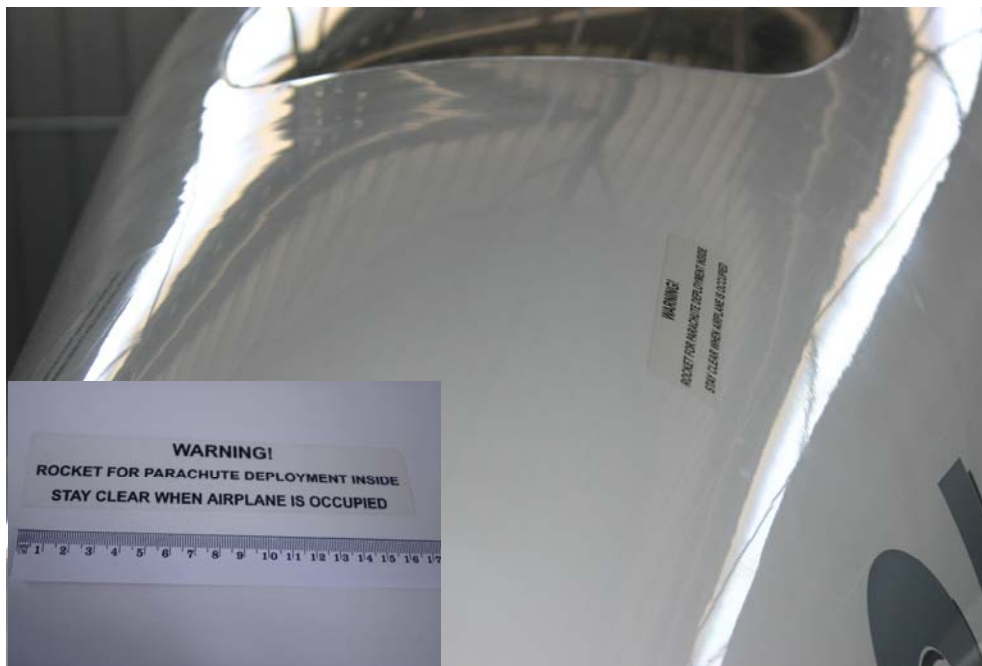
Figure 21: Typical fuselage CAPS warning placards
