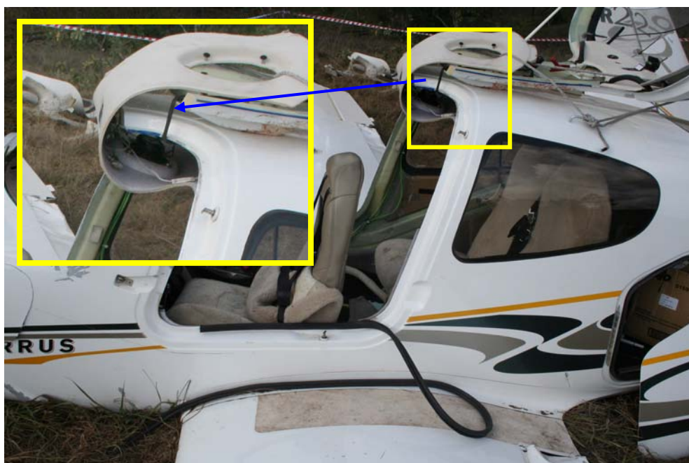
Figure 22: CAPS activation cable stretched tight on roof of aircraft.
