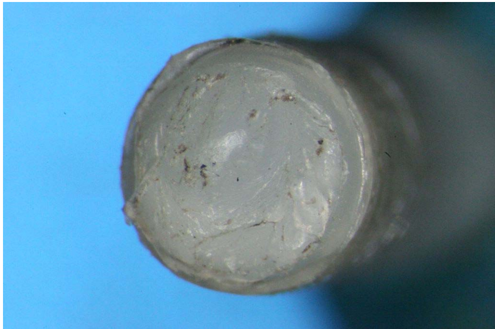
Figure 20: Fracture surface of nylon tension screw B
