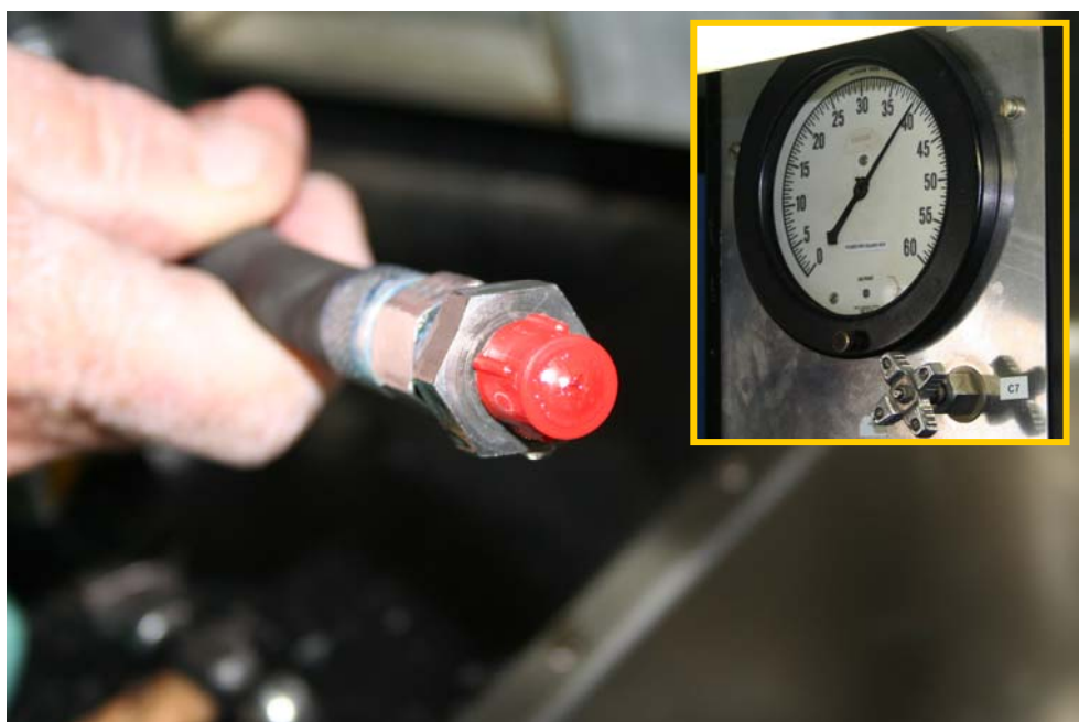
Figure 10: Pressure testing of the red plastic blanking cap from the accident site, with the gauge reading inset.
