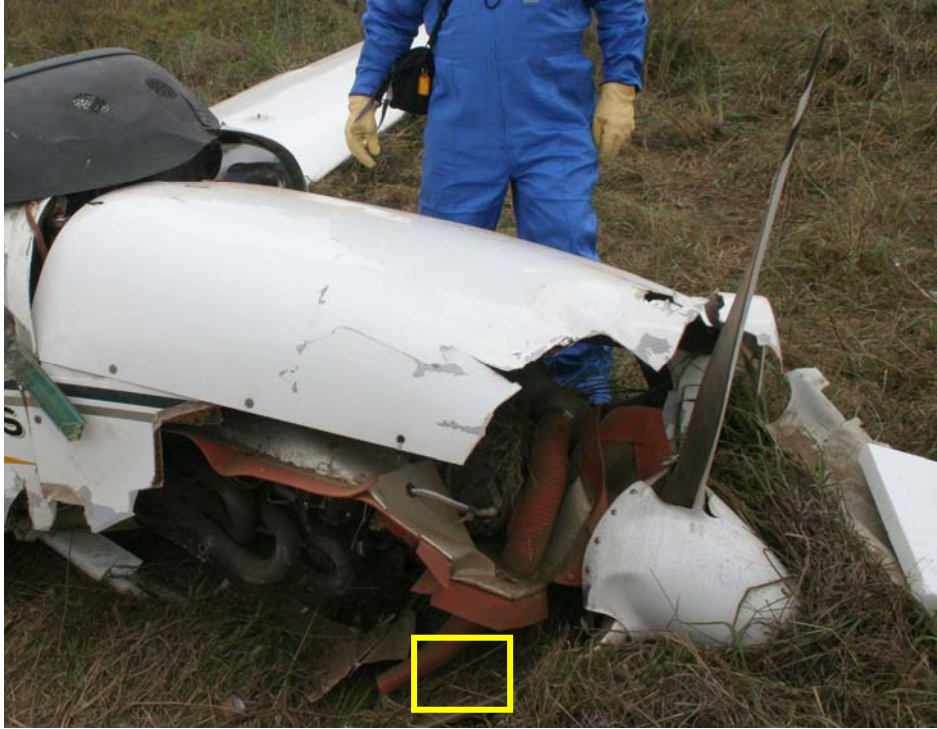
Figure 6: Detail of red plastic blanking cap location
