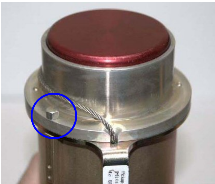
Figure 24: New design pick-up collar; showing aluminium tension screw (circled)
