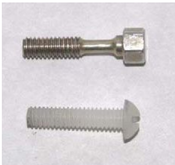
Figure 23: New design aluminium tension screws (upper) compared to nylon type (lower)
