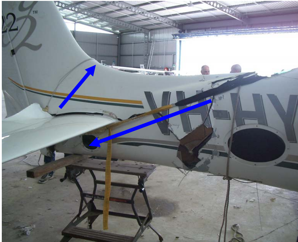
Figure 14: Path travelled by the CAPS rocket and harness
