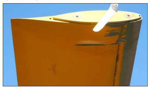
Figure 4: Damage to main rotor blade
