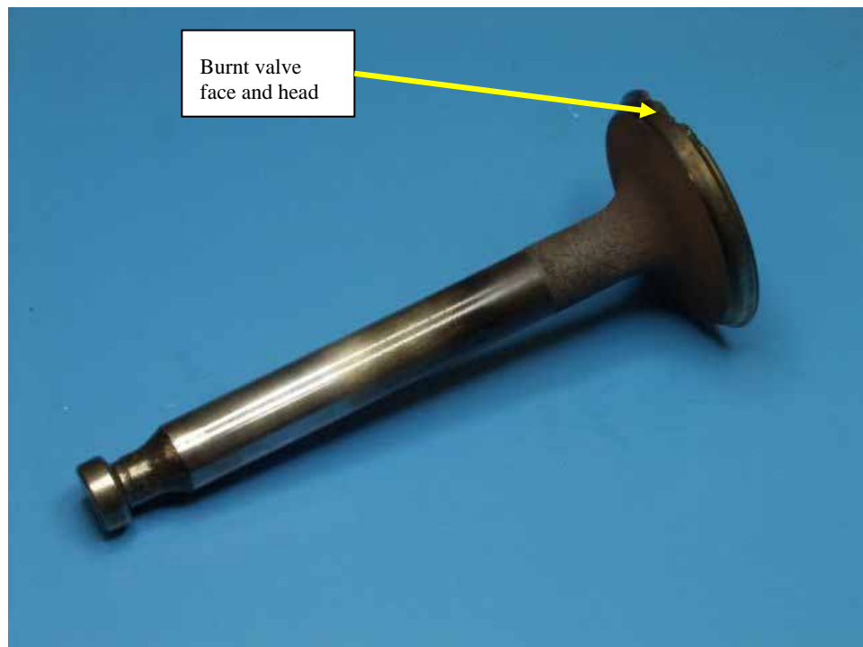
Figure 10: Burnt and worn left engine number-2 cylinder exhaust valve
