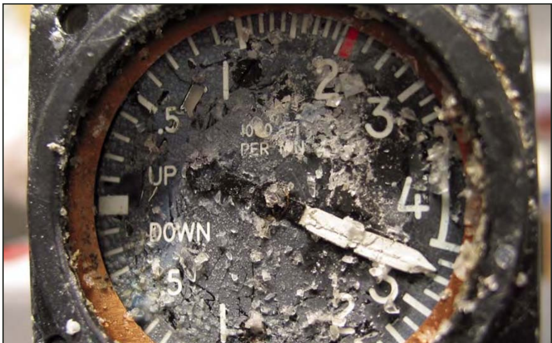
FIGURE 13: Vertical speed indicator
