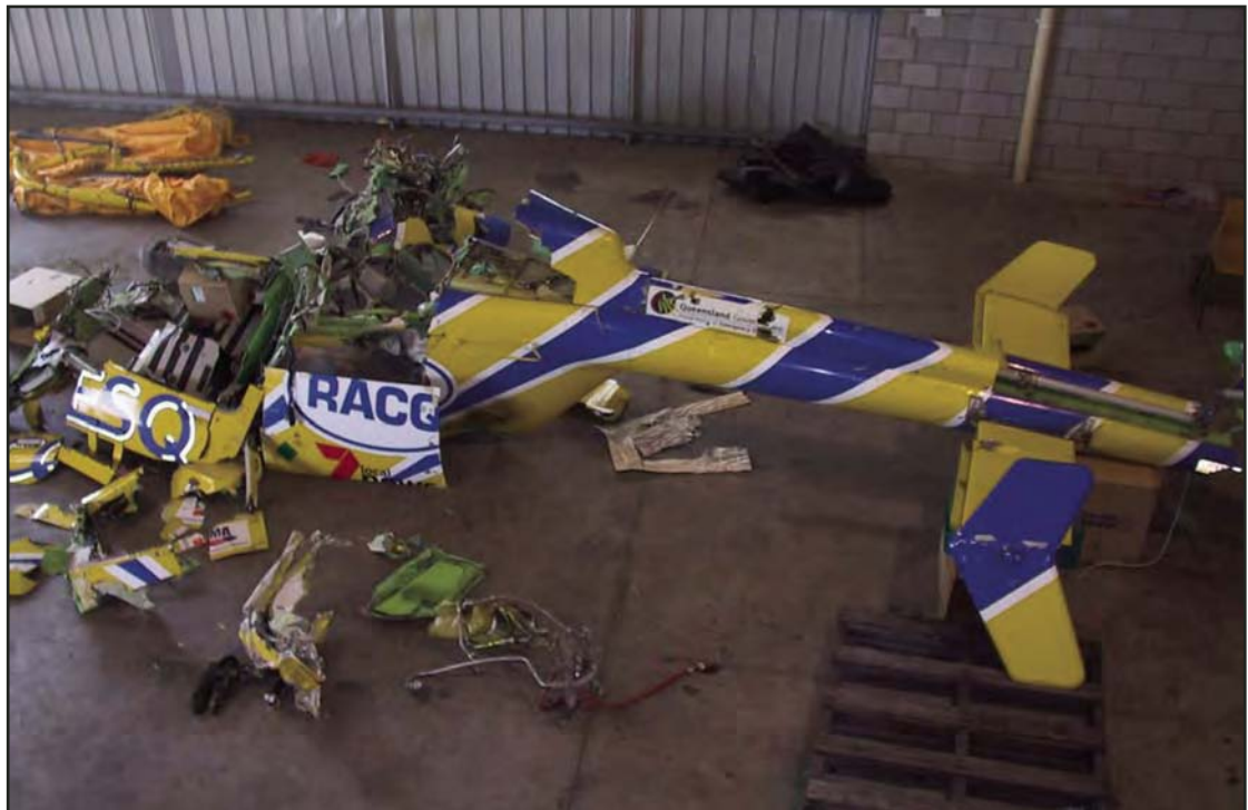
FIGURE 11: Reconstruction of the wreckage
