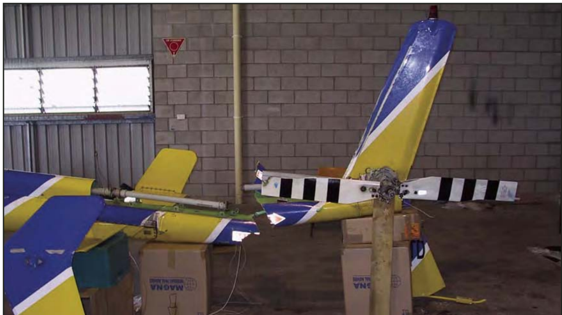
FIGURE 10: Tail rotor and separated tail section
