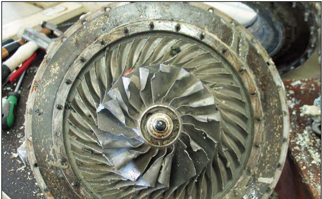
FIGURE 12: Engine compressor during disassembly
