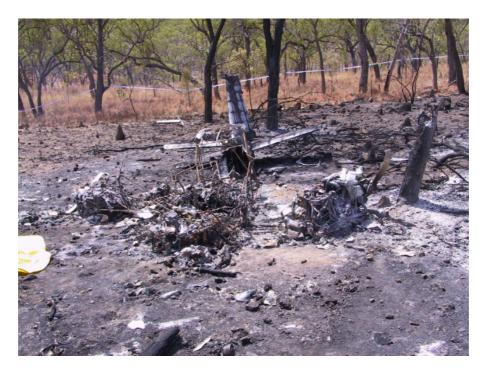
Although the engines were badly damaged by fire, a teardown inspection did not identify any evidence that either engine was incapable of delivering power prior to impact. A detailed examination of both propeller pitch change mechanisms indicated that both propellers were in the full fine pitch position at the time of impact.
