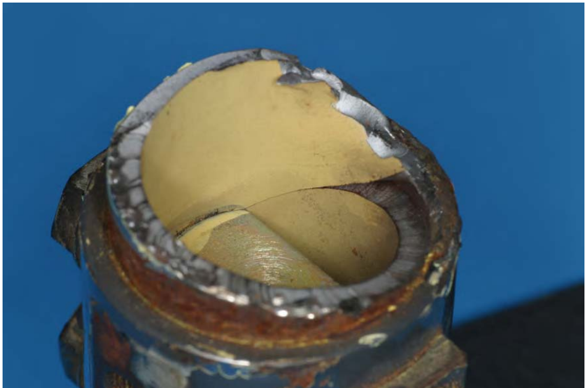
Figure 3. Shaft fracture surface showing the spiral form typical of torsionally induced failures.
