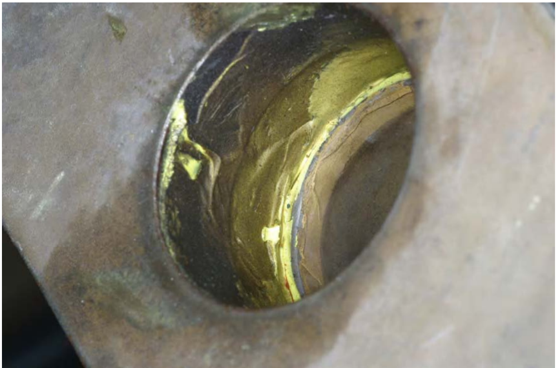
Figure 18. A soft jointing compound similar to that found on the failed shaft was observed within the comparison assembly.
