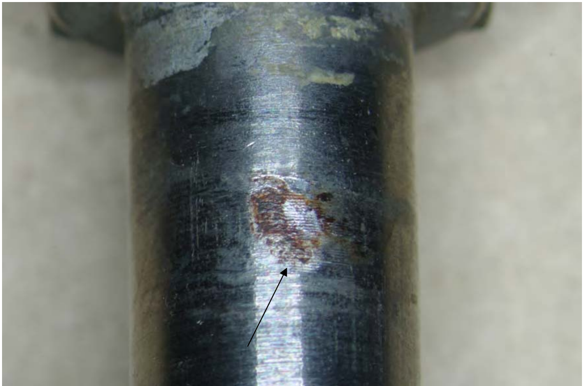
Figure 17. Bolt shanks from the comparison assembly also showed fretting damage and imprints from the hole machining.
