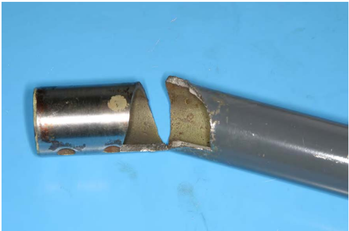
Figure 19. Fractured shaft sections from a previous (1992) failure. Note the similarity of the crack origin and propagation path.
