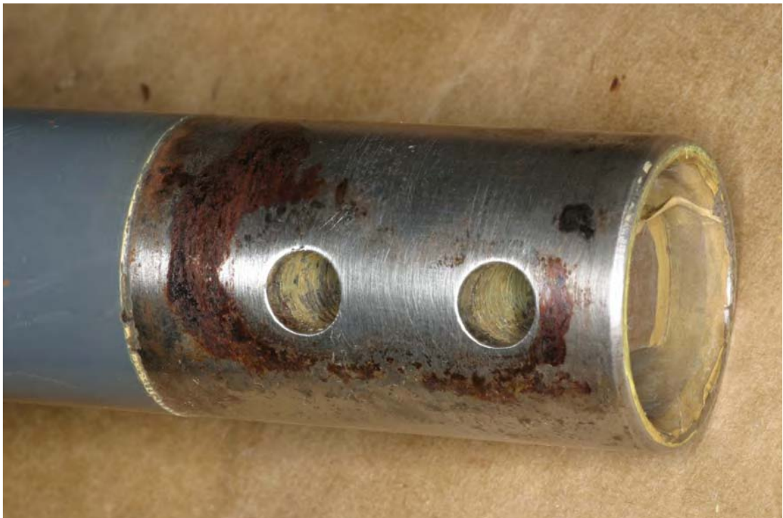
Figure 16. The surfaces of the clutch shaft from the assembly shown in figure 15. Fretting damage was also clearly evident.
