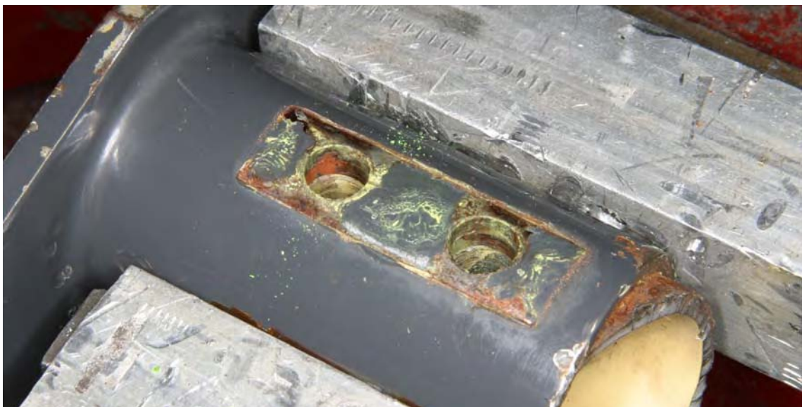
Figure 5. Removal of the bolt blocks revealed the assembly of the joint over the painted yoke surfaces.
