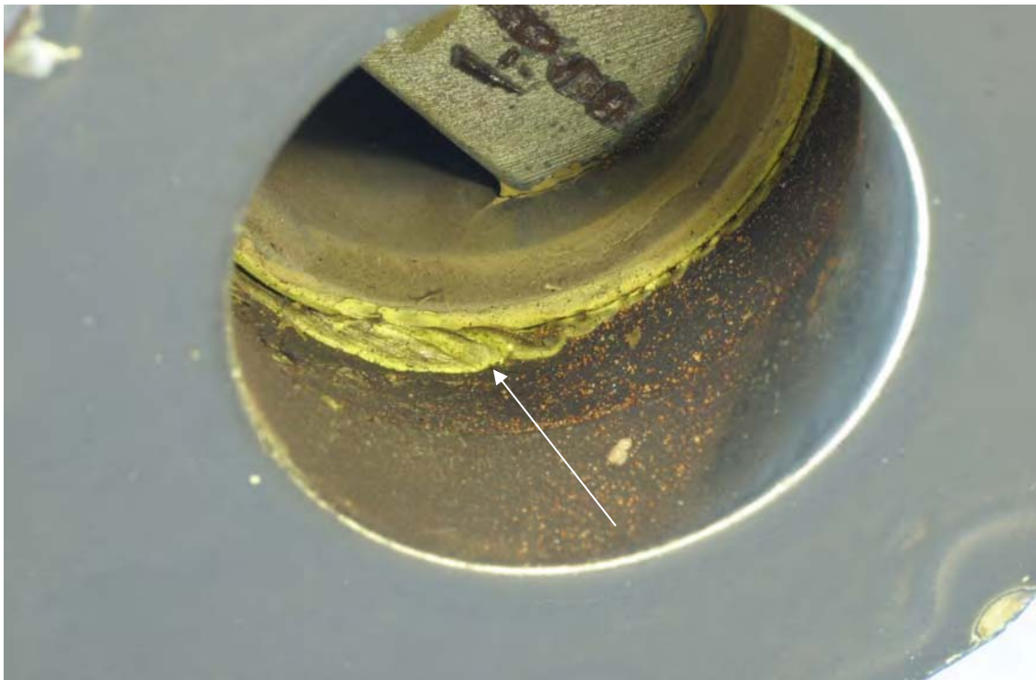
Figure 7. Arrow shows an accumulation of a soft jointing compound within the connection.
