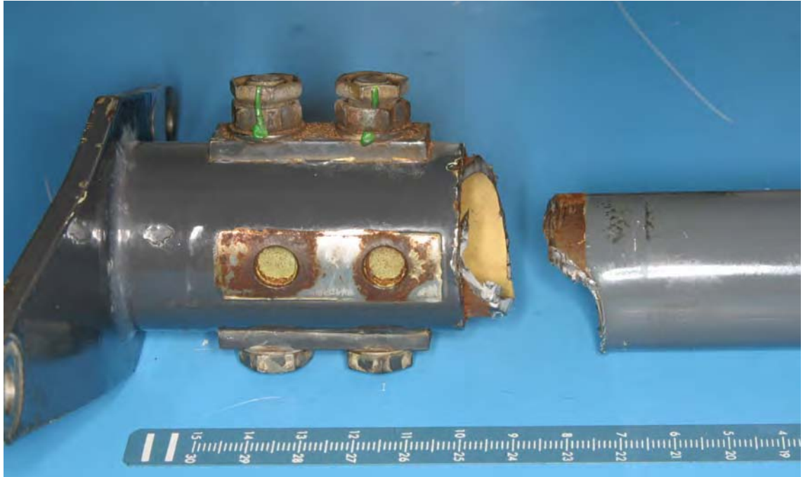
Figure 2. Clutch shaft, fractured at the point of connection with the flex-plate yoke.
