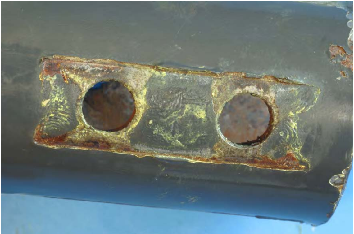
Figure 6. As shown in figure 5, the surfaces of the yoke had not been cleaned of paint before assembly of the clutch shaft connection.
