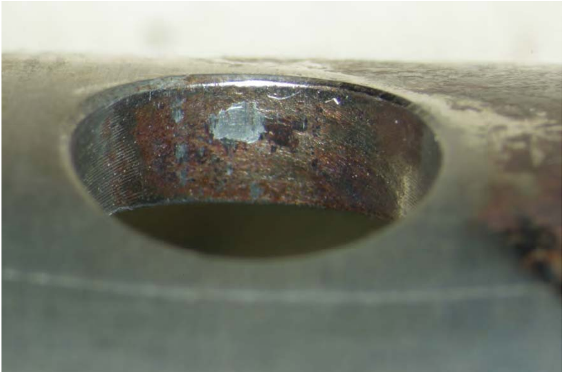
Figure 14. Fretting damage was also found inside the other clutch shaft bolt holes.
