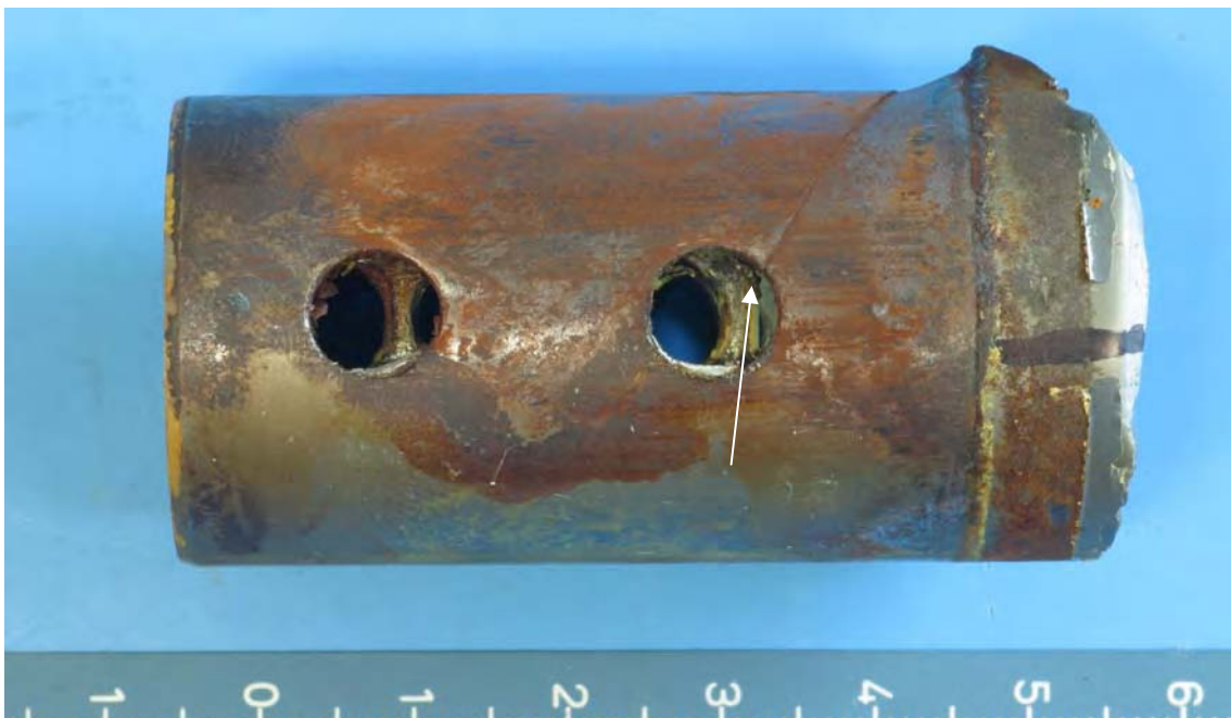
Figure 9. Stub of the clutch shaft removed from the yoke. Crack initiation point shown at the outer bolt hole. Also note the extent of fretting corrosion and damage from the joint movement.
