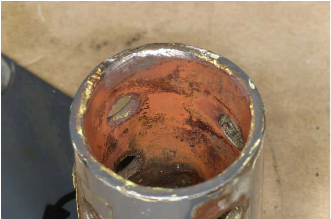
Figure 10. The inside surfaces of the yoke also showed extensive fretting corrosion.
