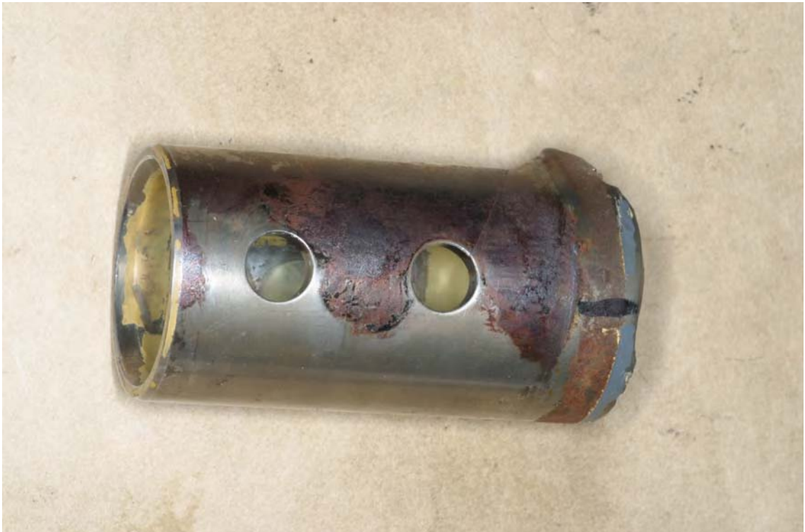
Figure 11. Removing the loose fretting corrosion product revealed the extent of the damage and the absence of any traces of zinc chromate or epoxy primer.
