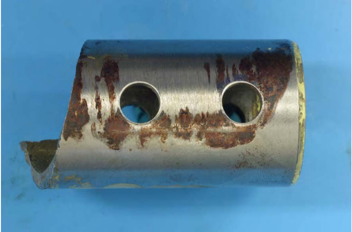
Figure 20. Extensive fretting damage was also evident on the interfacial surfaces of the previous clutch shaft failure.
