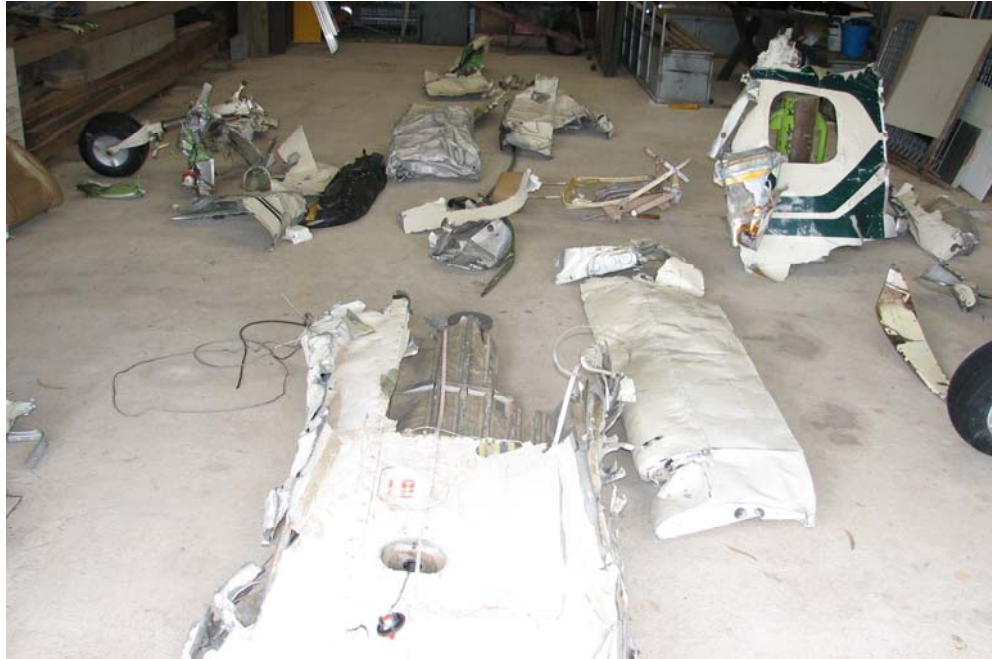
Figure 4: Wreckage loosely assembled in aircraft configuration
