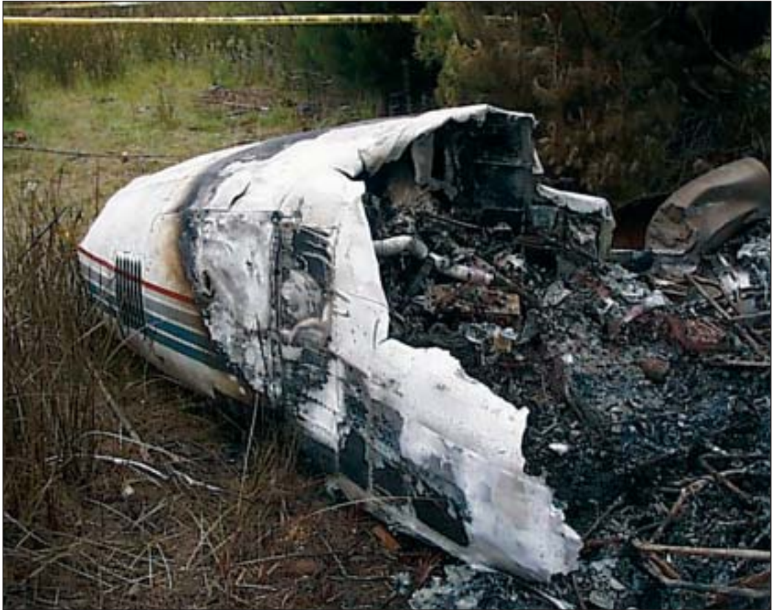
FIGURE 4: Extent of fire damage to cockpit area
