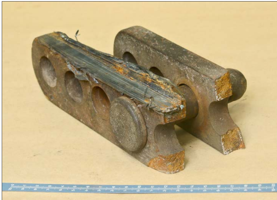
Figure A: General view of the broken end section from the compression rod as received by ATSB
