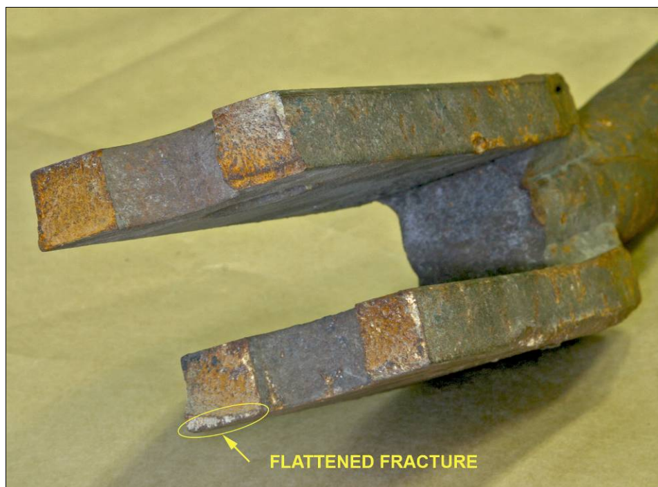
Figure 15: End view of the fractured surfaces of the compression rod
