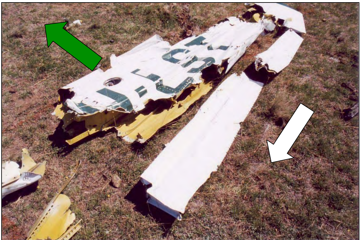
Figure 9: Separated left wing sections in reconstruction. Lower wing surface shown
