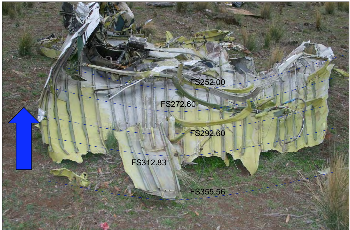
Figure 18: General view of aft fuselage flattened out left to right
