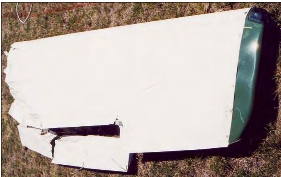
Figure 12: The separated right wing with the aileron reconstructed in the respective position
