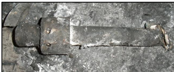
Figure 9: Failed connecting rod palm stud
