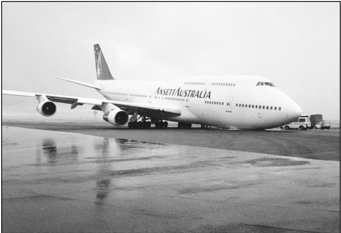
Figure 1. The aircraft on the runway with its nose-gear retracted.
