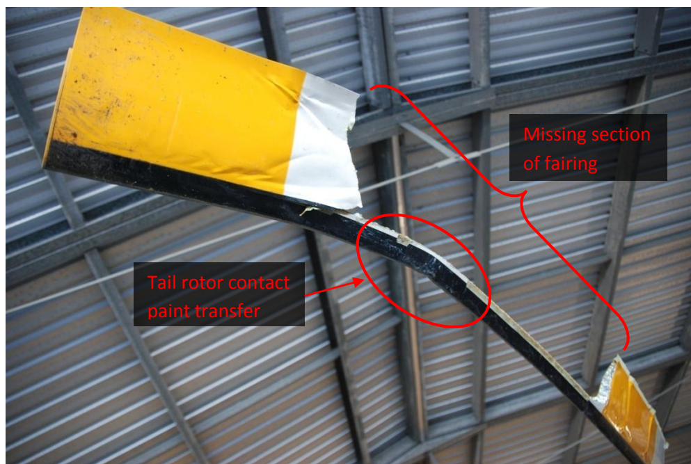
Figure 9: Main rotor blade, displaying forward bending and missing fairing
