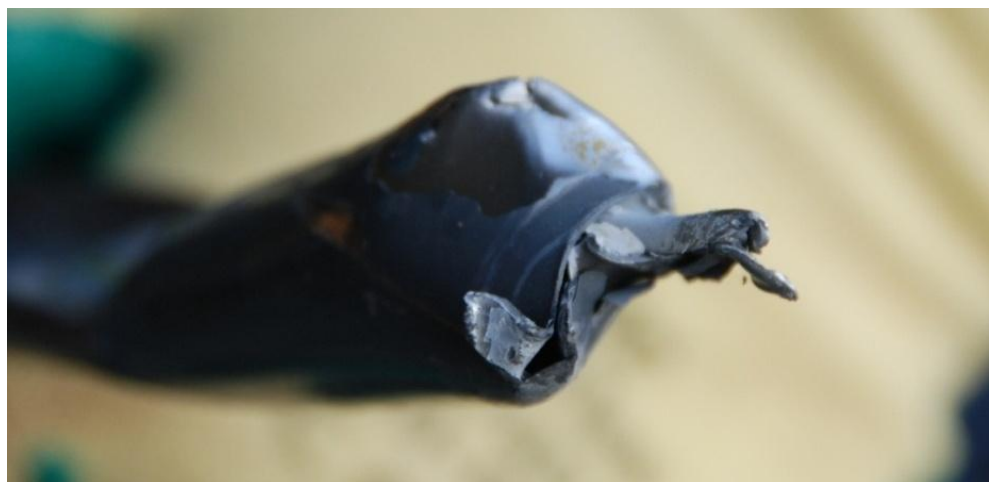
Figure 13: Tail rotor driveshaft with torsion damage
