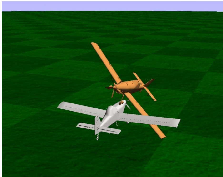
Figure 6: View of the derived relative position of ATB (grey) and CJK (bronze) at impact
