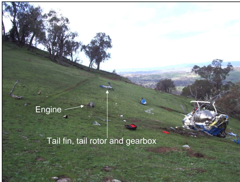
Figure 7: Rear structure impact damage
