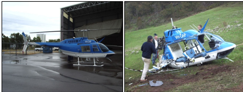
Figure 7: Rear structure impact damage
