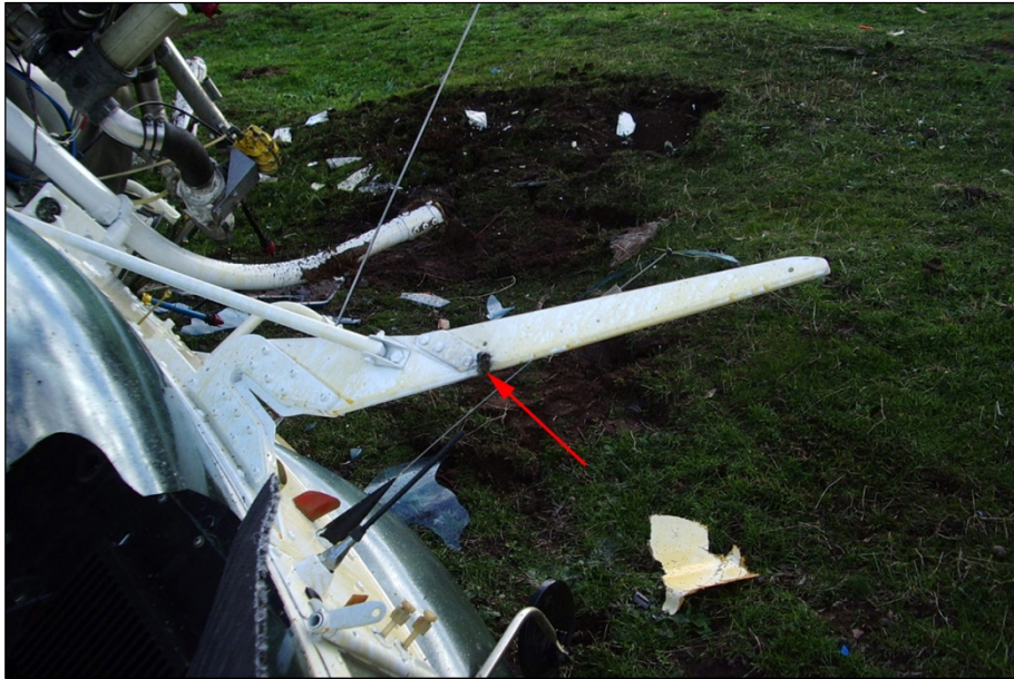
Figure 8: Penetration of the lower deflector by the wire
