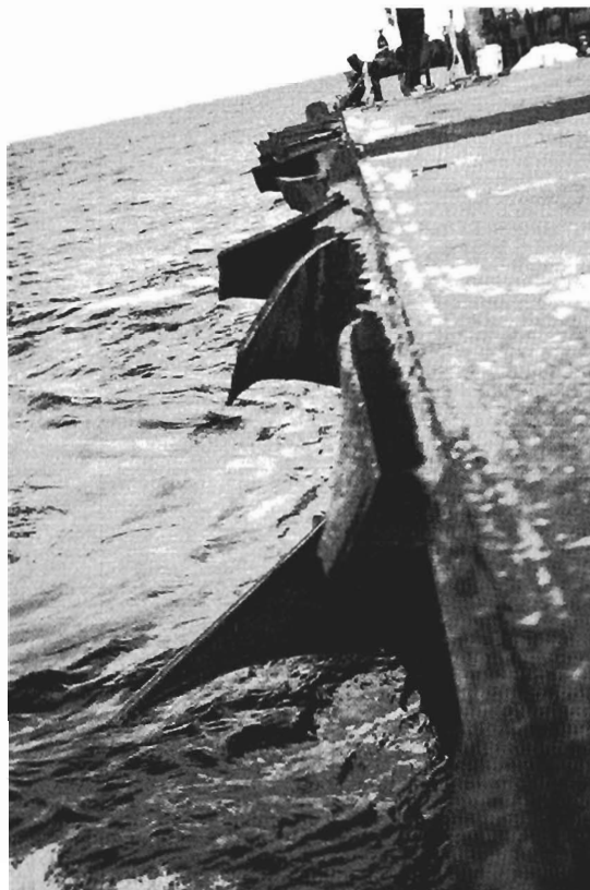
Photograph 4 View of fracture looking towards centre line from the port side
