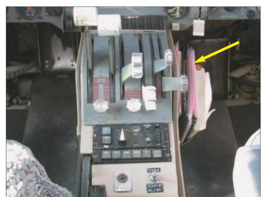
FIGURE 4: Location and condition of aircraft checklists
