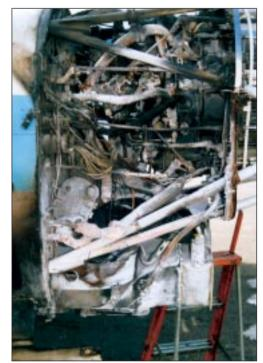
The starter generator, centrally located at the top of the engine compartment, sustained heat damage that melted the terminal block attached to the top of the unit, and the insulation on the feeder cables. The starter generator was not sooted.
