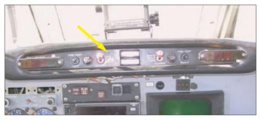
FIGURE 3B: Engine fire detection and extinguisher system panel
