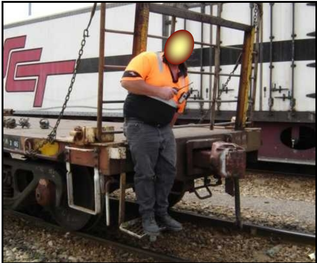
FIGURE 13. Illustration of shunter riding end step, (as at time of accident) facing forward holding radio. Practice now discontinued by SCT.
