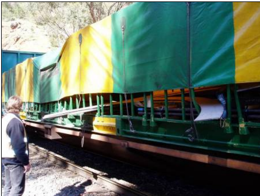
Figure 5: Photograph of shifted load
