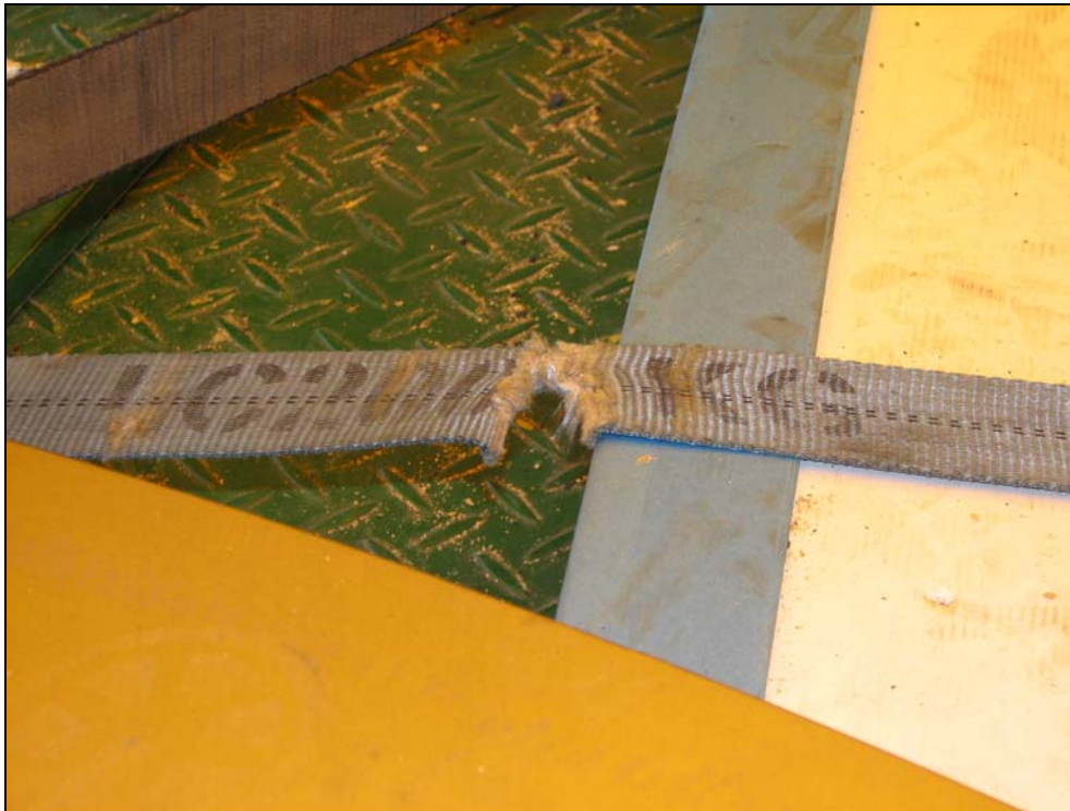
Figure 8: Damaged webbing strap
