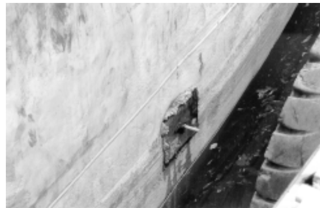
Temporary repairs effected to No 1 void space Figure 6
