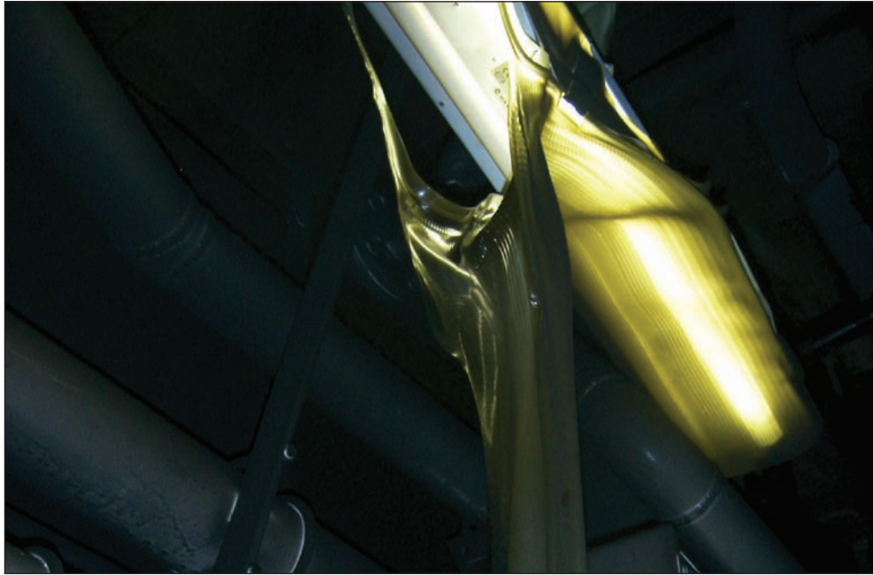
Figure 8: Melted light diffuser
