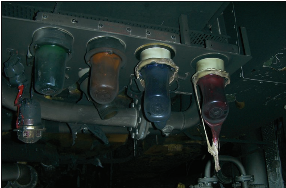
Figure 9: Melted alarm lights
