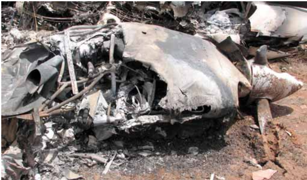
Figure 6: Left engine showing broken propeller blade
