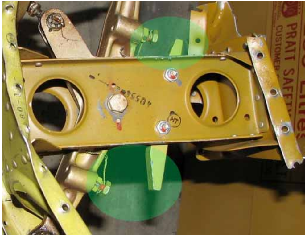
Figure 14: Right aileron stops showing absence of repetitive contact
