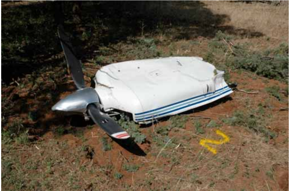
Figure 7: Separated right engine
