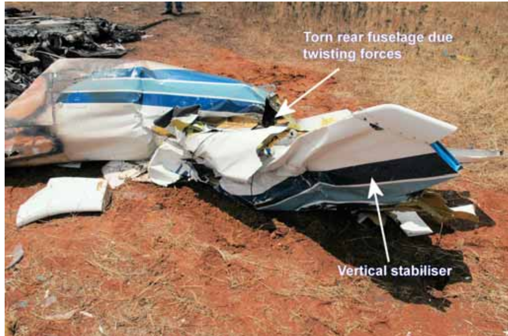
Figure 9: Torsional twisting to rear fuselage and empennage
