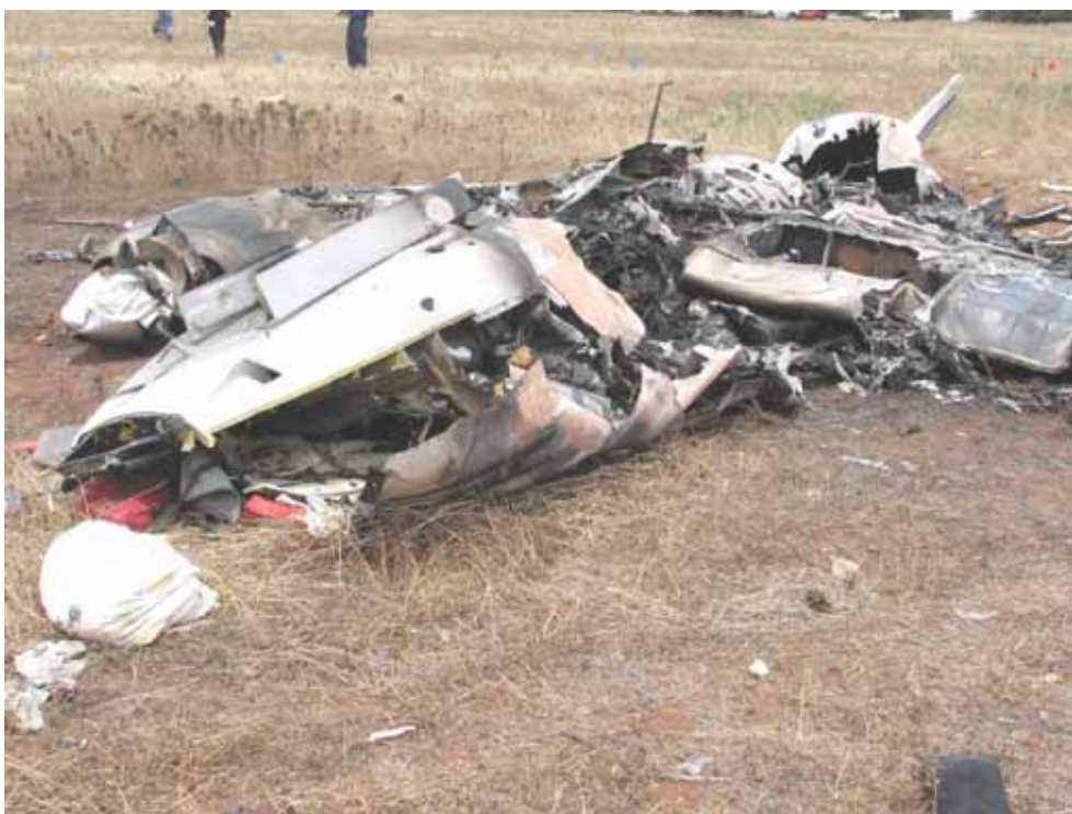
Figure 2: Burnt, inverted fuselage and inner wing sections
