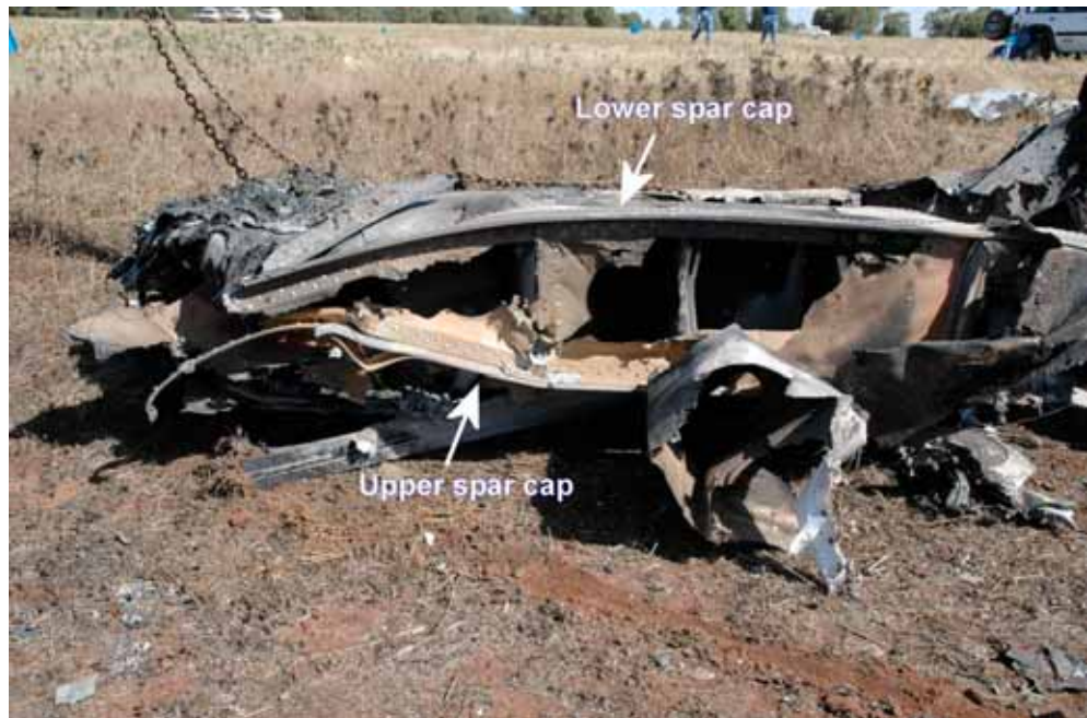
Figure 8: Failed left wing main spar (inverted) outboard of engine nacelle
