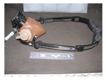
Both crew members found that the elastic strap fitted to their masks was not tight enough to provide an adequate positive seal of the mask against their face, resulting in the need to physically hold the mask against their face to obtain effective oxygen flow. A random check of these types of masks, fitted to another operator's aircraft also found that the elastic straps had been stretched to a point where the mask was no longer held tight on the user's head.
