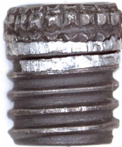
Figure 3: Close view of one of the threaded inserts showing 'stripped' thread material from the heat exchanger
