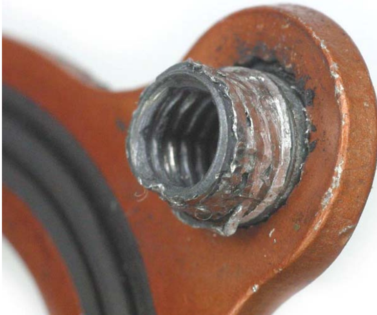
Figure 5: Opposite view of the insert from Figure 4, showing it had been pulled completely through the gasket
