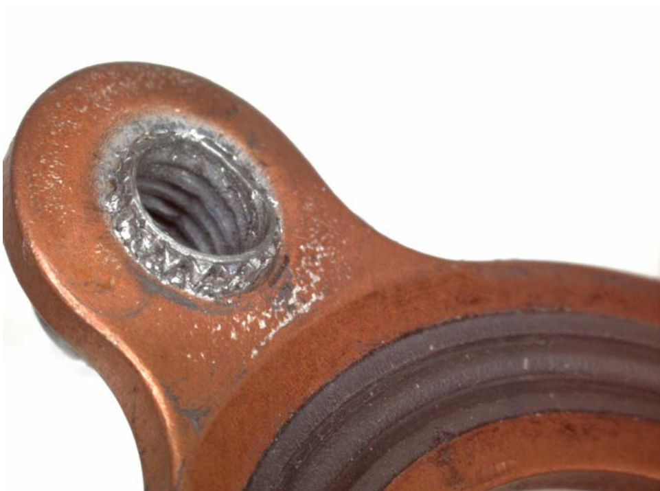
Figure 5: Opposite view of the insert from Figure 4, showing it had been pulled completely through the gasket
